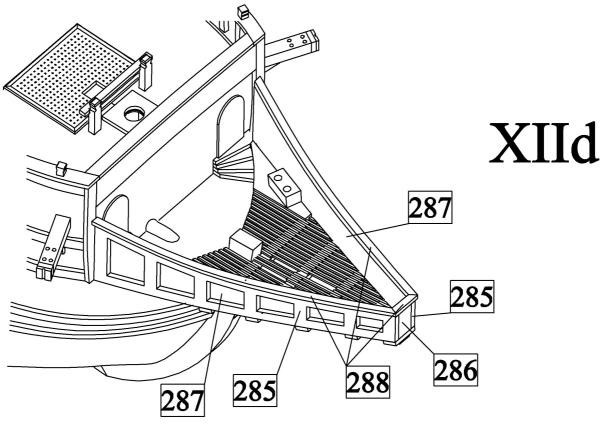
e) First glue beams 191 and cross beam with belaying pins 126 to the side of head railing. Then grind by sand paper bowsprit from dowel and tie it to the head by rope 195 as it is shown in the figure.
