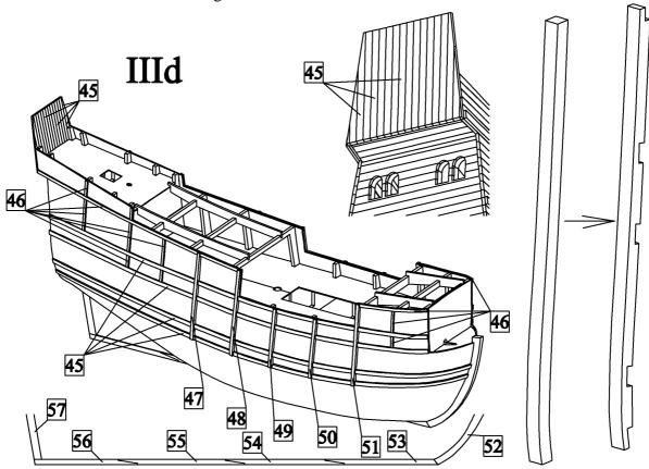
e) Carefully cut off parts of the frames which overhang the decks.
