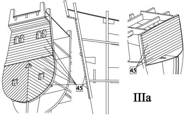
b) Glue first reference strip to the skeleton. The position of the first plank is shown in the plan. Glue the strips in direction from bow to stern.
