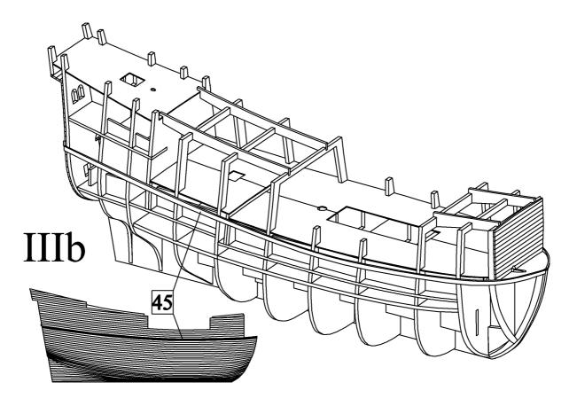
c) Planking the whole hull. Glue the strips again in direction from bow to stern. It needs to grind some strips (mainly in the lower section of the hull) into required shape so that would fit well.
