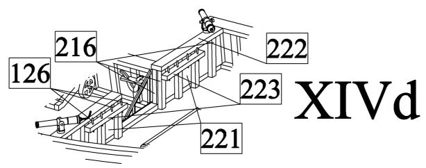
e) Glue cross beam 220 with belaying pins 126 to the railing on forecastle deck.
