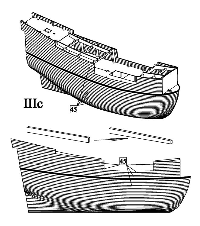
d) First planking the stern. Then glue keel and stem and sternpost (parts 52-57) to the hull-start with part 52 and then stepwise other parts in direction from 53 to 57. Then glue wales 45 and 46 to the hull. Finally glue reinforcements 47-51 to the hull. It is need to grind by needle file slots as it is shown in the figure.
