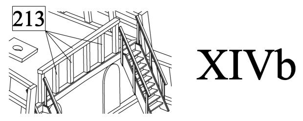
c) Make railing on quarter deck from parts 215-215. Then glue cross beams 219 with belaying pins 126 to the railing.
