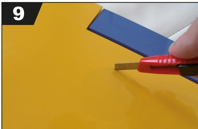
Use a hobby knife with #11 Blade to cut the covering from the area above the aileron servo mounting position.
