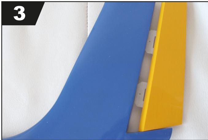
Glue the hinges in the rudder with 5 min epoxy. Align the rudder to the fuselage and glue it with 5 min epoxy.
