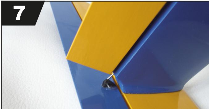
Cut a small rectangle according the form of the elevator horn in the elevator and glue it with epoxy.
