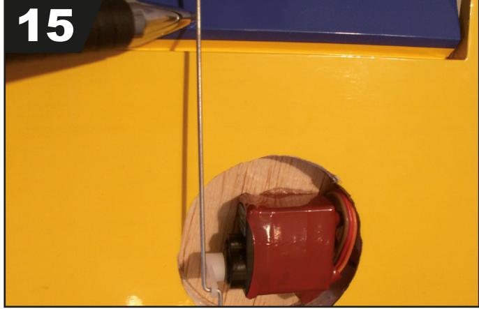
Install the aileron pushrod and align it to the aileron. Mark the position.
