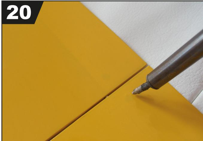
Use a knife or soldering iron to open the holes for the wing mount screws. Glue the aluminium sleeves.
