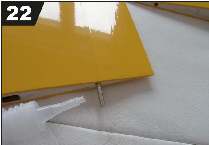
Glue the center pin and wing joiner in one wing
