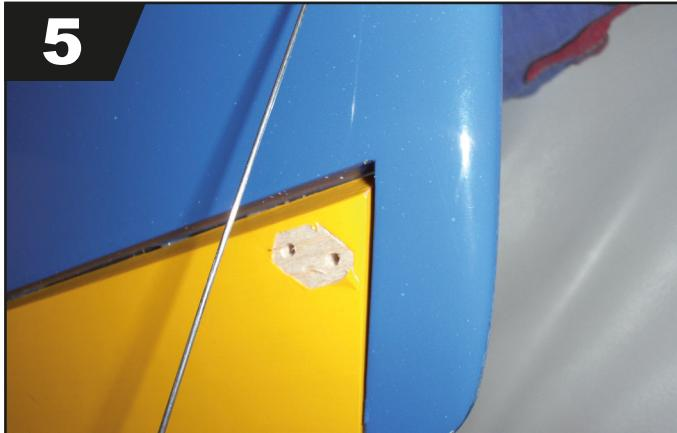
Ad light pressure to the pushrod and bend them towards the rudder and mark the position of the rudderhorn. Use a 2mm drill for the holes and remove the cover before you glue the servo-horn with CA.
