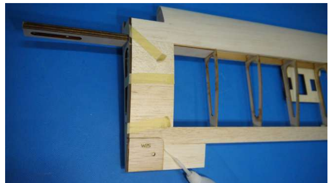
Line up W28 and W24 and attach the back edge and side with instant glue, then attach W25 with instant glue.
