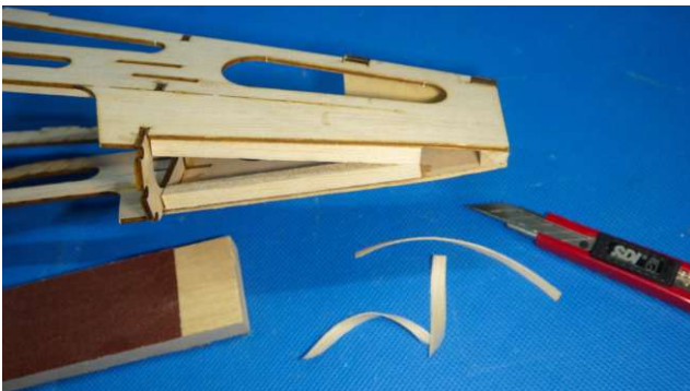
Sand and cut off extra pieces of balsa wood.
