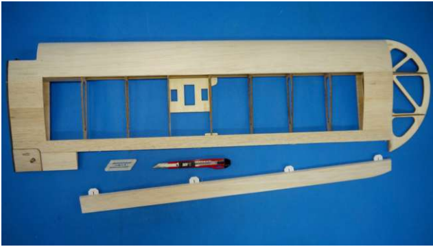
According to aileron, cut hinge holes.
