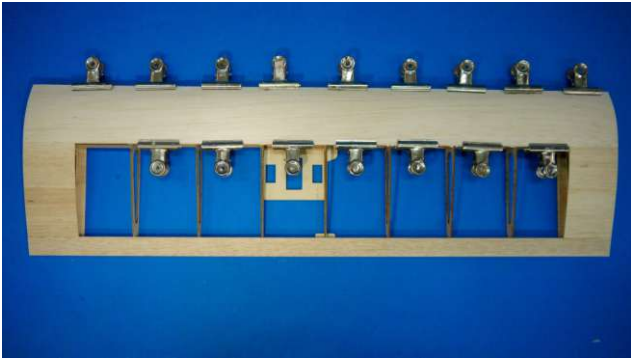
Cover with covering. Secure with clips.
