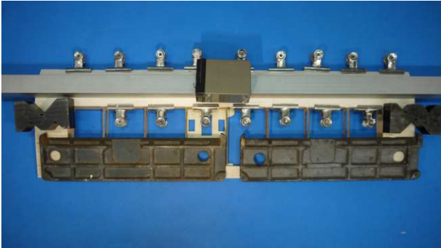
Clip to secure and immediately use weights to hold down the covering until the glue has dried.
