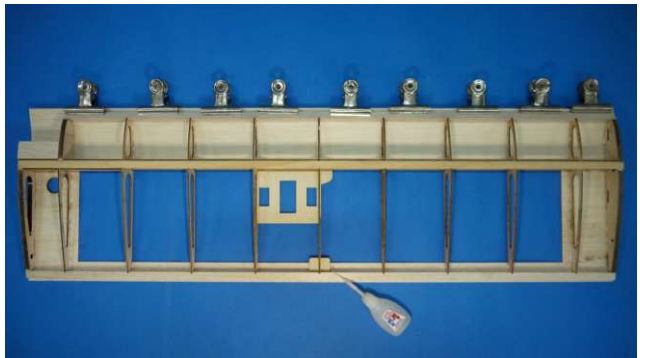
The hole must be on the wing root side.
