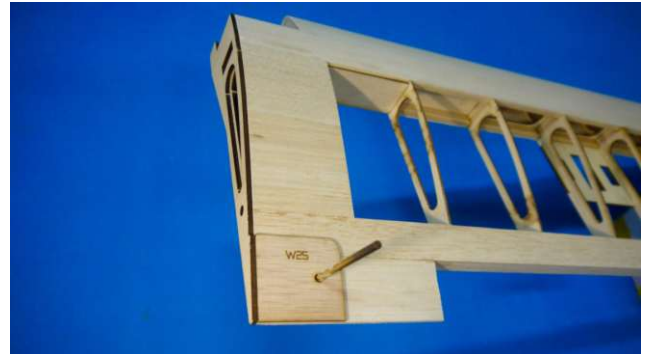
According to W25's hole, drill a 4mm hole.
