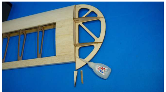
Attach W21, W22 and W23 with instant glue. Prepare two pieces of W27.
