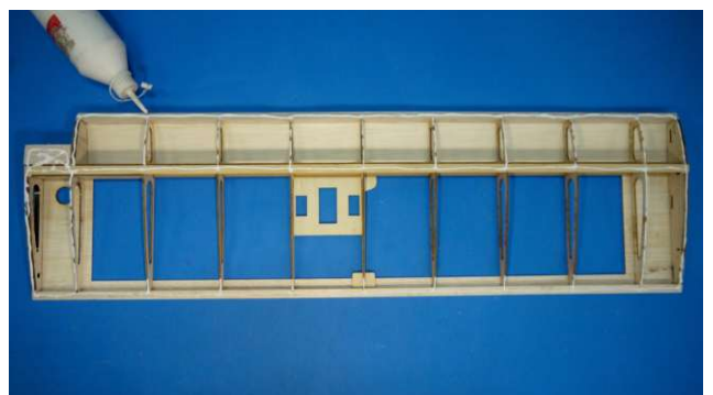
Apply white glue to all wing ribs and upper surfaces. Note: This should be done on the upper side of the wing.
