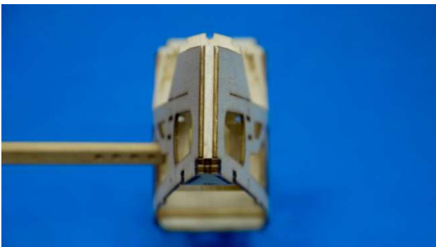
Rear view of the fuselage. Make sure it has bilateral symmetry.
