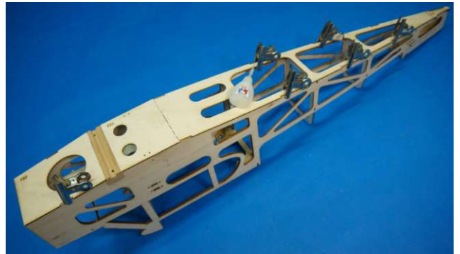
Attach F20 and F21, and secure with clips.
