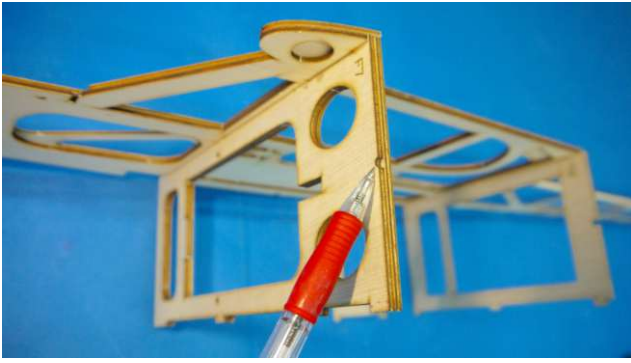
F7's mark should be facing toward the nose of the plane.
