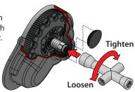
high-pitch, whining noise. Remove the rubber slipper clutch plug on the transmission cover in order to adjust the slipper. Use the 4-way wrench to turn the adjusting nut clockwise to tighten and counterclockwise to loosen. Place the model on a high-traction surface, such as carpet. Adjust the slipper so that you can hear it slip for approximately two feet from a standing, full throttle start. (Learn more about adjusting the slipper clutch in the sidebar left.)
