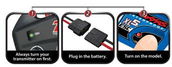
Always use new or freshly charged batteries for the radio system.
