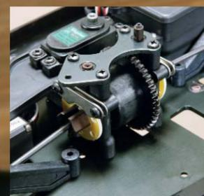
The center diff is supported by an aluminum brace. The hardened-steel spur has beveled teeth, and the phenolic brake discs are excellent.
