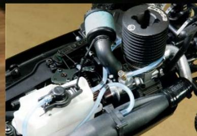
A composite tuned pipe expels the exhaust. I think that the 125cc fuel tank might have been a bit small for the large engine, which drank the fuel rather quickly.
