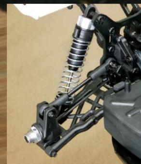
The rear suspension uses the same arms as the front and is flipped side to side. This minimizes the need for a bunch of different spares. The plastic-body shocks are very smooth and do a great job of absorbing jumps and bumps.
