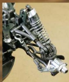
The cast-aluminum steering blocks look strong enough to endure any mishaps. The linkages are adjustable (but they aren't turnbuckles!).
