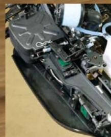
The radio gear is tucked away in a box with a rubber boot over the on/off switch. A one-piece plastic radio tray holds the high-torque metal-gear servos that function superbly.
