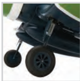
Impressive landing gear. Retractable, 90° rotating electric main landing gear (installed)
