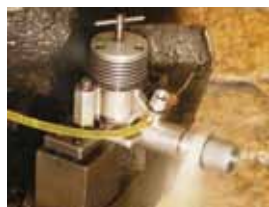
Standard PAW 15GTS on test showed easier compression setting and needle adjustment
