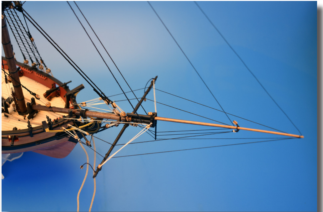
Above Main topmast stay and preventer stay. The collar and mouse at the mast head end is set up as the lower mast stays, except the 'mouse' is the smaller F-18. Below - Fore topmast stay and preventer stay. The ends of the stays run through the 'bees' near the bowsprit cap and down to the forecastle, where they are set up with blocks and tackle, as shown in the line drawings on the plans.
