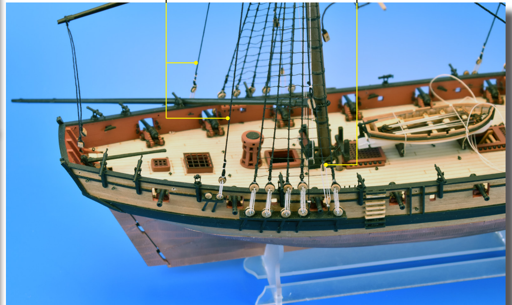
Above and below - Before adding the topmast stays, rig the topmast back stays
