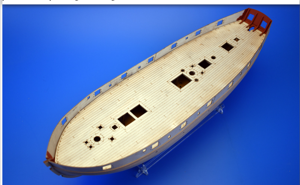
20 - Dry fit the deck (128) before committing to glue. Sand any edges that may not fit perfectly. It does not matter so much if the deck edges are slightly short of the bulwark edges as the inner bulwark planking will hide any slight gaps. Once the deck fits as it should, use PVA wood glue to fix the deck in place, plus a few brass pins along the near edges to ensure the deck sits flush with the false deck.
