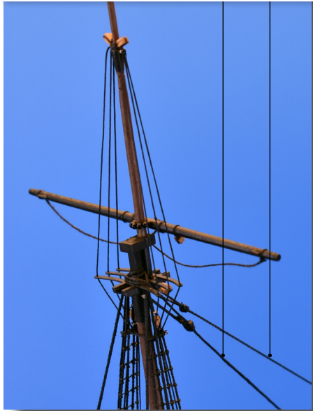
Above Main topmast stay and preventer stay. The collar and mouse at the mast head end is set up as the lower mast stays, except the 'mouse' is the smaller F-18. Below - Fore topmast stay and preventer stay. The ends of the stays run through the 'bees' near the bowsprit cap and down to the forecastle, where they are set up with blocks and tackle, as shown in the line drawings on the plans.
