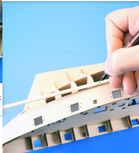
Below - Marking out the taper starting position at the stern.
