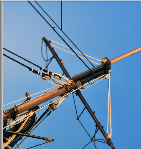
Above Main topmast stay and preventer stay. The collar and mouse at the mast head end is set up as the lower mast stays, except the 'mouse' is the smaller F-18. Below - Fore topmast stay and preventer stay. The ends of the stays run through the 'bees' near the bowsprit cap and down to the forecastle, where they are set up with blocks and tackle, as shown in the line drawings on the plans.
