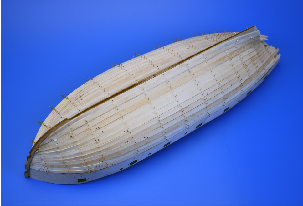
First planking complete. Remove all brass pins and sand the hull smooth using coarse followed by medium grit abrasive paper. A small electric sanding mouse would make the sanding quicker and easier, but be very careful at the extremities, as it is very easy to damage the stem at the front, or go too far at the stern.
