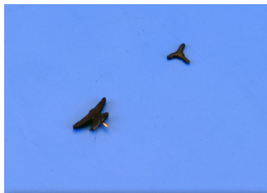
Bulwark cleats. Paint the photo etched cleat (PE-30) and larger laser cut cleat (89) black. Insert a pin through the middle of part 89 to help secure it in place.
