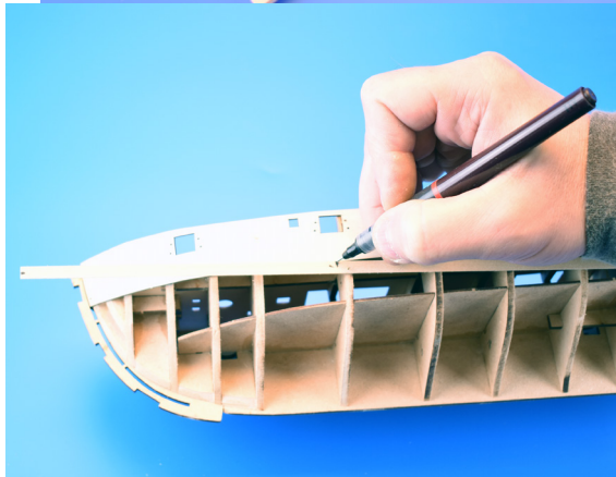
Above - marking the taper starting position onto the plank. When the plank overlaps the gun port pattern, mark out and taper this area.
