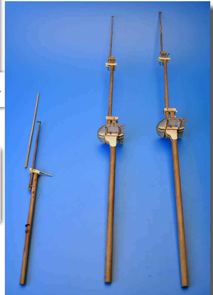
Fore and main topgallant masts showing the lower ends with main caps in place, followed by the 'fids' or stoppers.
