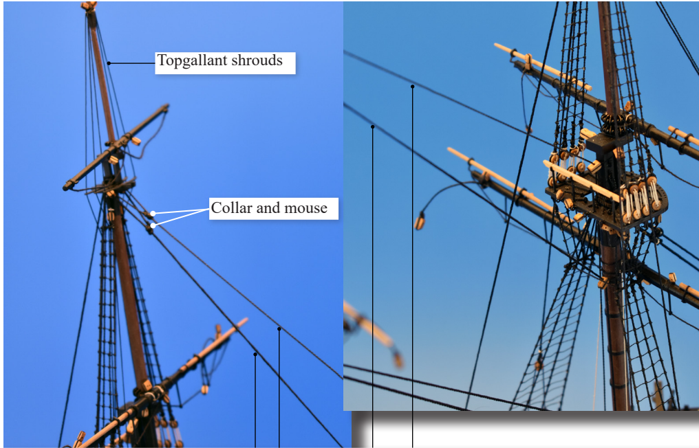
Above Main topmast stay and preventer stay. The collar and mouse at the mast head end is set up as the lower mast stays, except the 'mouse' is the smaller F-18. Below - Fore topmast stay and preventer stay. The ends of the stays run through the 'bees' near the bowsprit cap and down to the forecastle, where they are set up with blocks and tackle, as shown in the line drawings on the plans.
