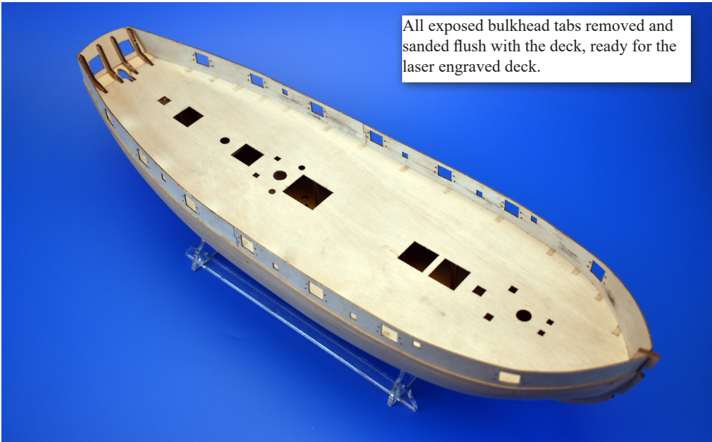
20 - Dry fit the deck (128) before committing to glue. Sand any edges that may not fit perfectly. It does not matter so much if the deck edges are slightly short of the bulwark edges as the inner bulwark planking will hide any slight gaps. Once the deck fits as it should, use PVA wood glue to fix the deck in place, plus a few brass pins along the near edges to ensure the deck sits flush with the false deck.
