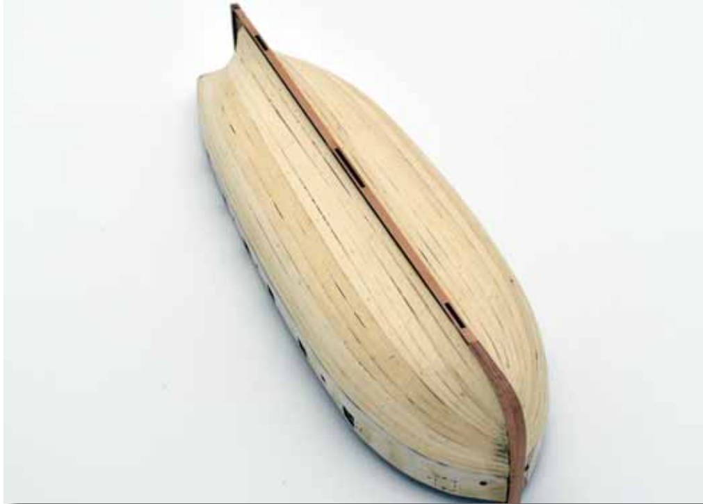
50. Add the outer stern counter pattern (122) using PVA wood glue and clamps to keep firmly in place until set. The picture above shows part 83 temporarily clamped into position, to help gauge the correct positioning of 122.
