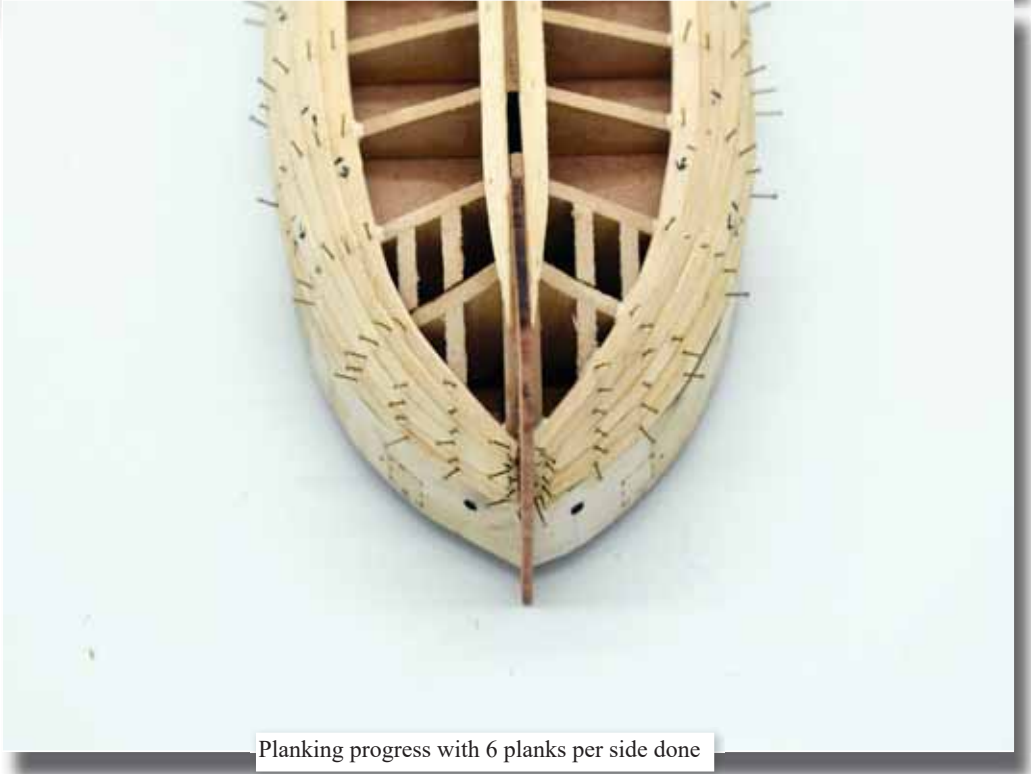
The taper position marks can be clearly seen in this picture.
