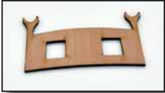
74. Remove the stern transom (83) from the 1.5mm wood sheet and glue in place, as shown. Again, this can be clamped until the glue has cured. Once cured, file the openings so both layers are completely flush with one another.
