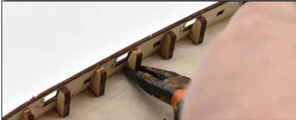
63. Remove all bulkhead tabs above deck level by carefully bending and twisting with a pair of pliers or similar. Once removed, sand any remaining stubs flush with the deck.
