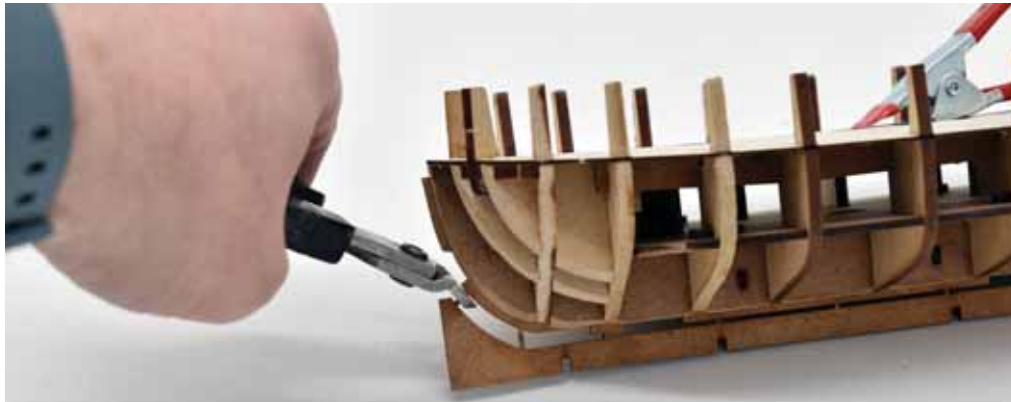
35. Now that the hull structure is strong and rigid, the spacer jig can be removed. Cut the tabs close to the keel using side cutters, followed by filing the remaining stubs flush with the edge of the keel.
