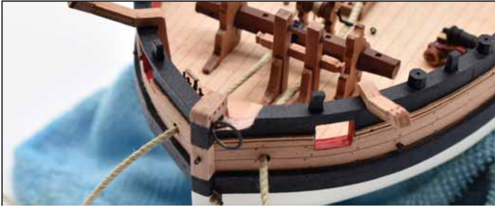
129. Once the area has been rounded enough for the bowsprit to fit through, PE-5 can be slotted in place as shown
