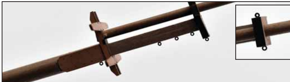
126. Using the plans, mark out, drill and insert the eyelets to the positions shown.
