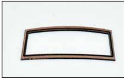
76. Remove the stern transom framing (83a) from the 0.8mm wood sheet and glue in place, as shown. You can use either PVA wood glue and pin in place or cyano glue.
