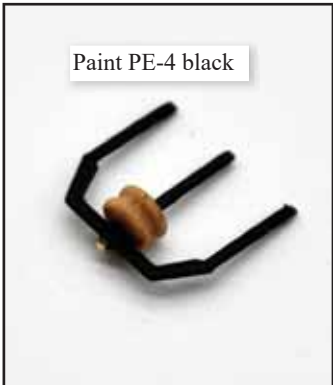
114. Make up the sheave assembly that is fixed to the left hand side of the prow, using PE-4 and a 2.5mm sheave. Slot into the position shown. Also drill and insert an eyelet to the end of the prow as shown.
