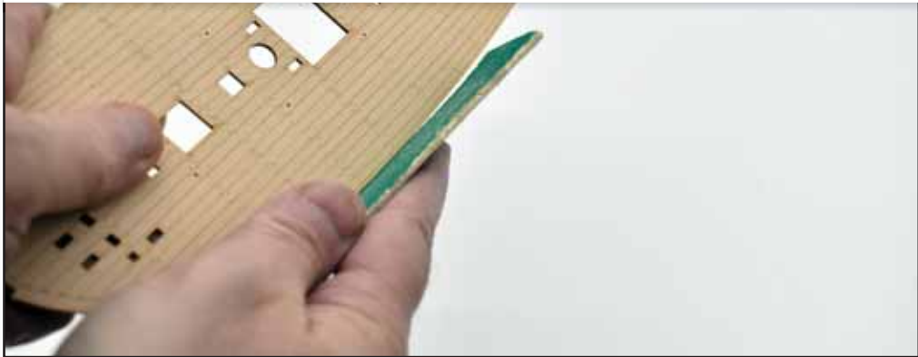
64. The laser engraved 1mm lime wood deck is now ready to be glued in place. Trial fit the deck and sand/file (below) any tight spots around the edges. Because there is another 'spirketting' plank that covers the inner bulwark, it does not matter if there is a slight gap between the deck edge and the bulwark sides.
