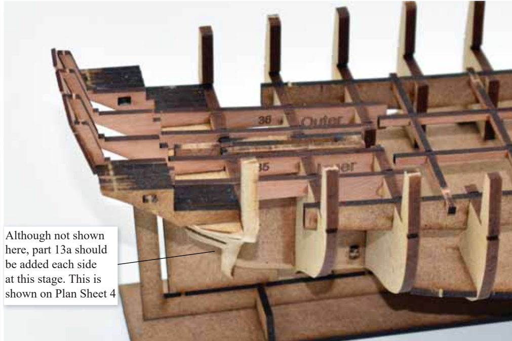
28. Glue parts 24 and 24a to the outer stern frame (36), using 24a to lock the parts and align correctly
