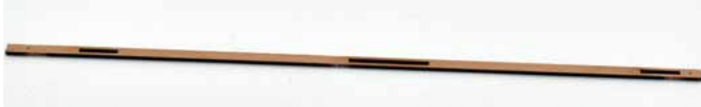
48. The main keel (33) can now be added. Pin as well as glue into position, making sure the slots for the drop keels line up with the slots in the hull
