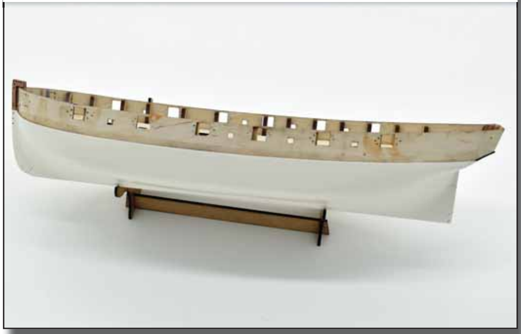
59. Hull painting fully complete and all masking removed. Touch up any areas that require attention
