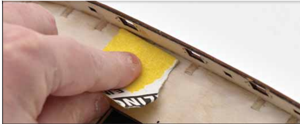
63. Remove all bulkhead tabs above deck level by carefully bending and twisting with a pair of pliers or similar. Once removed, sand any remaining stubs flush with the deck.
