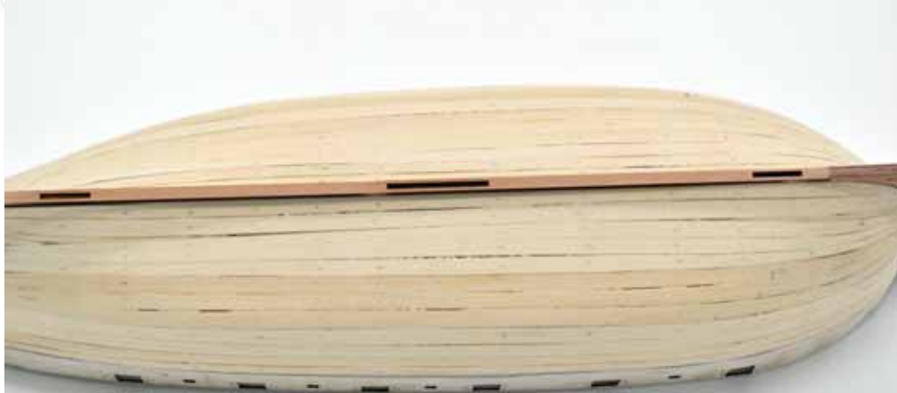
48. The main keel (33) can now be added. Pin as well as glue into position, making sure the slots for the drop keels line up with the slots in the hull
