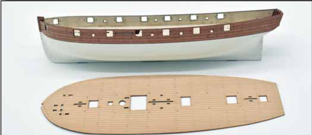
64. The laser engraved 1mm lime wood deck is now ready to be glued in place. Trial fit the deck and sand/file (below) any tight spots around the edges. Because there is another 'spirketting' plank that covers the inner bulwark, it does not matter if there is a slight gap between the deck edge and the bulwark sides.
