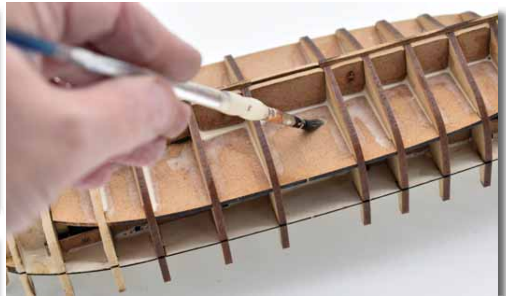
36. To further strengthen the hull assembly, you can brush on watered down PVA wood glue under the lower and upper decks.
