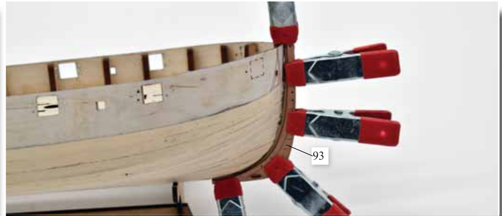
46. Add the outer facings to the prow, 93 right and 94 left. Use K-3 to lock the parts in place and PVA wood glue to fix. Clamps are shown, securing the assembly until the glue has cured.
