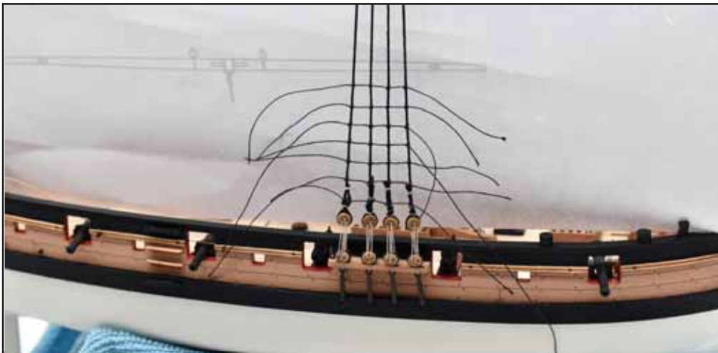
139. It is now time to add ratlines. These ratlines will run parallel to the waterline. As a guide, the lines are approximately 6mm apart. When the lines are installed, brush some dilute PVA over the knot and allow to dry properly. NOTE: Please try NOT to add any tension to the vertical lines as that will pull them out of shape and distort them.
