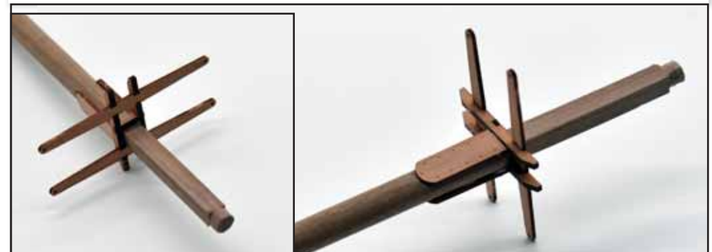
122. Using the plans for dimensions, make up the main mast. The upper part is to be square, and the very top round, to fit the mast cap.
