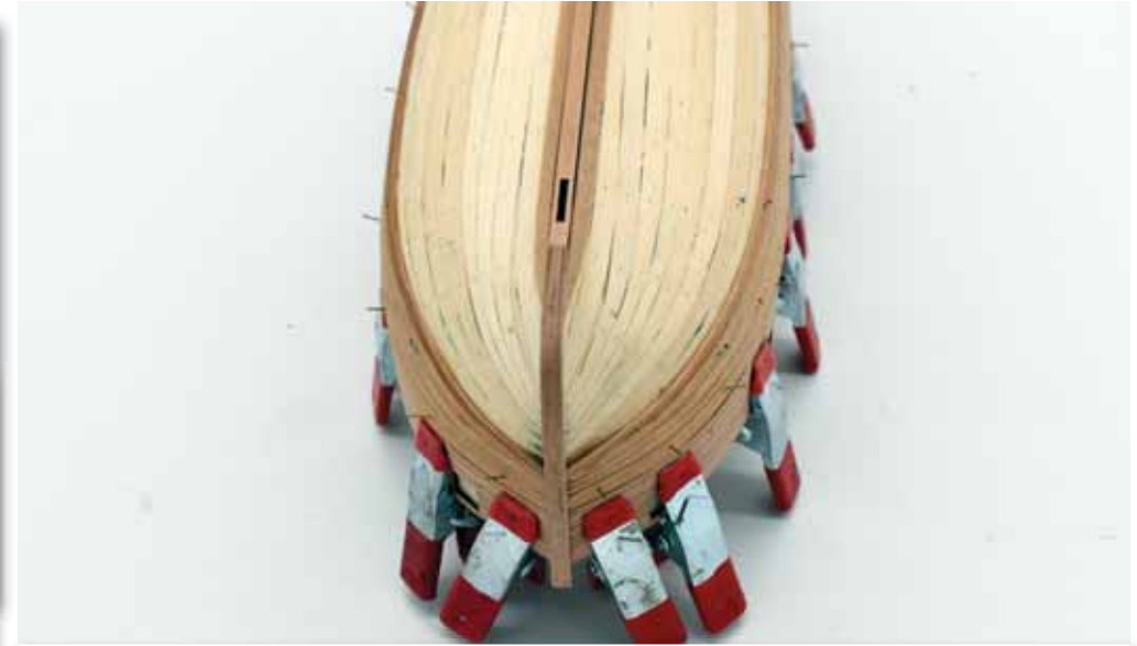
Planking progress at bow (above) and stern (below). If you do not get the end planks at the stern perfectly butted up against the stern counter, do not worry too much, as this line is covered by stern counter rails (124 and 125)
