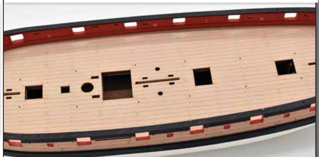
78. Carefully glue the gunwales in place so there is more or less an equal overhang on the outer and inner bulwark sides. You can use cyano glue or PVA and pins. If the latter, you can do the same as the main wales, and pin in place, and then cut off the tops of the pins flush with the top surface of the gunwales, and then re paint black.
