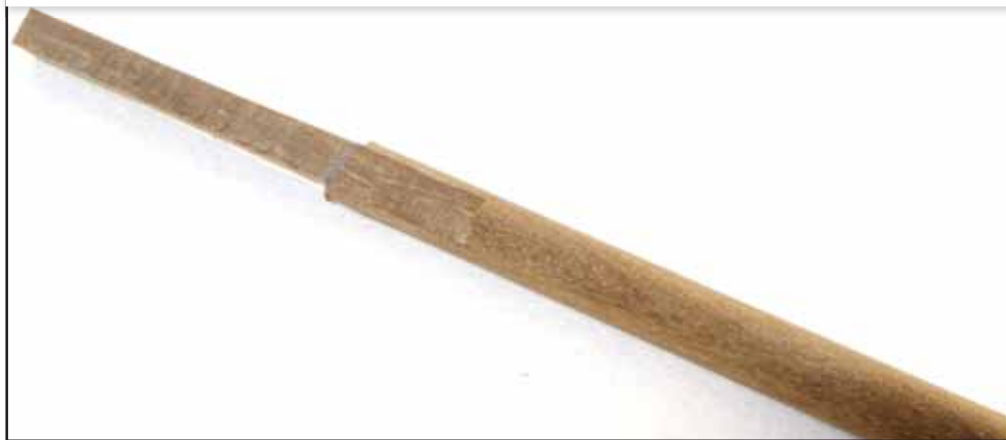
308. Shape the lower mast sections as shown and on plan. This will take some time to take your time here.
