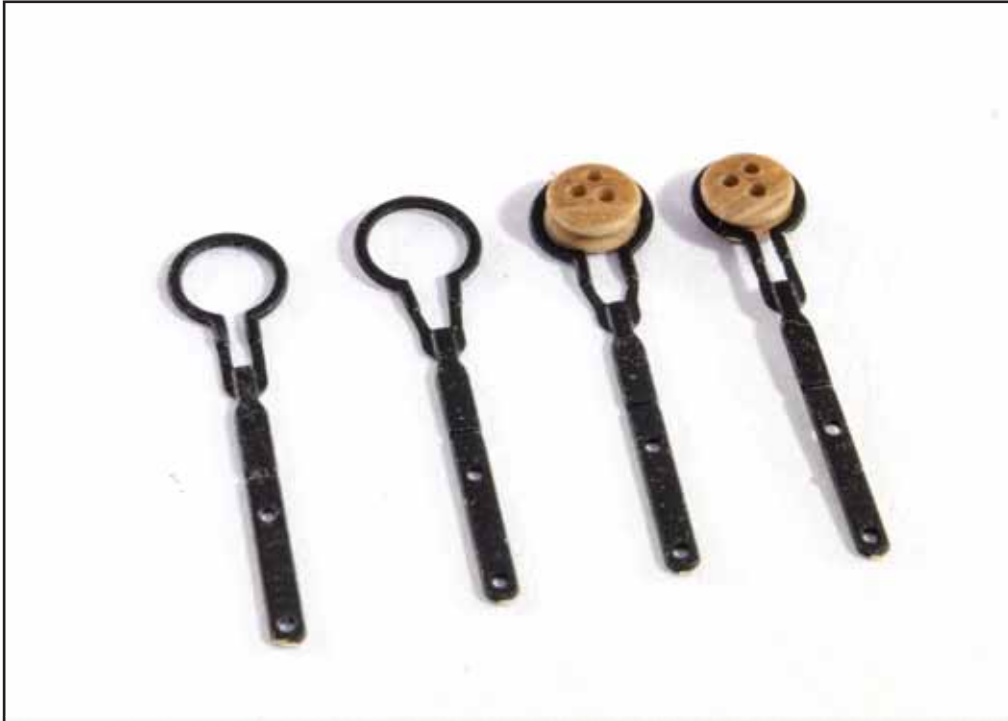
285. From the 0.4mm PE sheet, remove parts PE-28. Slightly prise open the loop, sit a 4mm deadeye within the loop, and then close the loop again.
