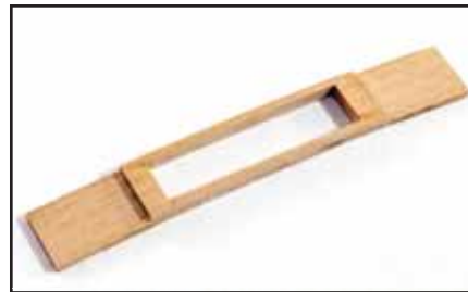
131. Your assembly will look like this. Gently sand the lowest concave edge, slightly bevelling it from the front, towards the back. This will allow for the angle of the deck.
