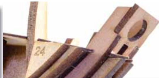
63. Glue into place. The bevelled edge will sit against the deck.
