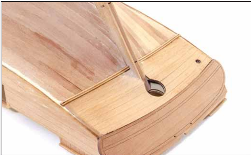
134. Glue these as shown. These fit along the edge of the second planks, just up to the line where the counter is glued. The hole on each of these will sit on the outside edge.
