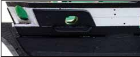
143. Round the edges, especially on the underside of parts #62. Paint these black and glue into place as shown.
