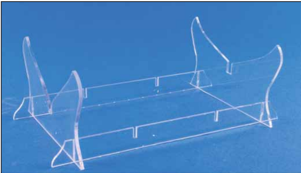
334. Lastly, remove all parts from the acrylic sheet and remove the protective backing film. Take the pieces shown here and assemble. You can use a little glue here if you wish, but if you use CA, make sure you use the type which doesn't cause fumes.
