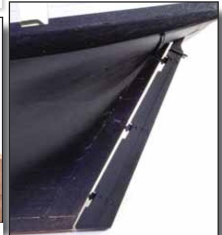
152. Temporarily install the rudder to the hull as shown.
