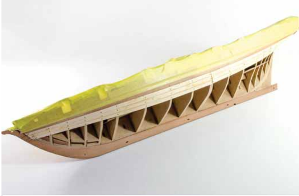
96. Continue to plank the hull, tapering as you go. You will find it beneficial to start tapering the planks from around the double bulkhead point as you progress. No tapering needs to be done at the stern.
