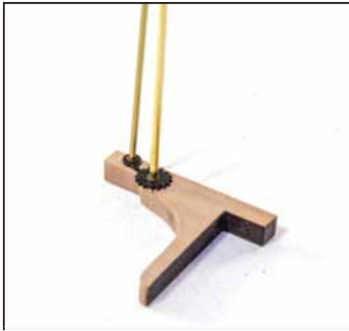
222. Use a length of 1mm brass rod, slide it through PE-20 gear and slot into the lowest hole as shown. Take a length of 0.8mm brass rod, slide it through the pawl PE-21 and insert into the upper hole. Don't glue.
