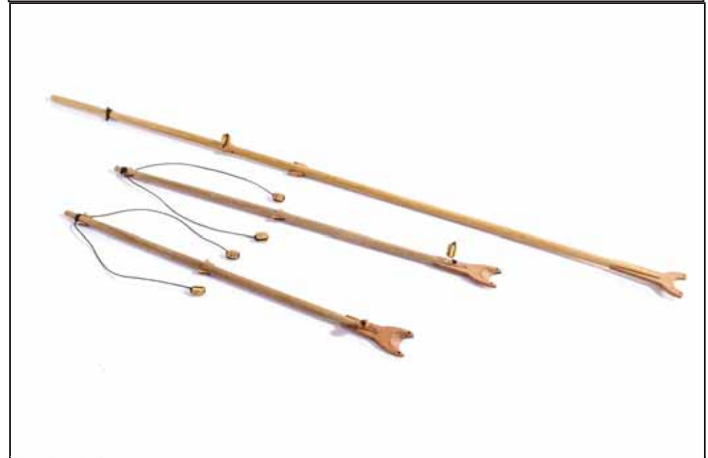
323. You must now take build all of the remaining timber parts from the mast/rig plans. All of these can be painted black either before or after fitting out with blocks etc.
