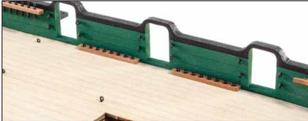
177. We have supplied a small bag with some 1.5mm black balls. These are the cannon shot, and you can drop these into the shot garland holes as shown. Again, carefully brush a little varnish over them to glue them down.
