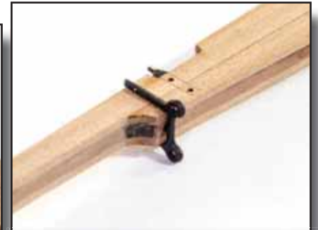
150. Drill a 1mm hole in the rear of the rudder and fit PE-6 as shown here, using CA.
