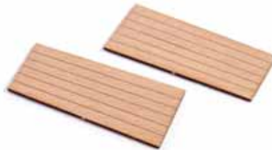
131. Your assembly will look like this. Gently sand the lowest concave edge, slightly bevelling it from the front, towards the back. This will allow for the angle of the deck.
