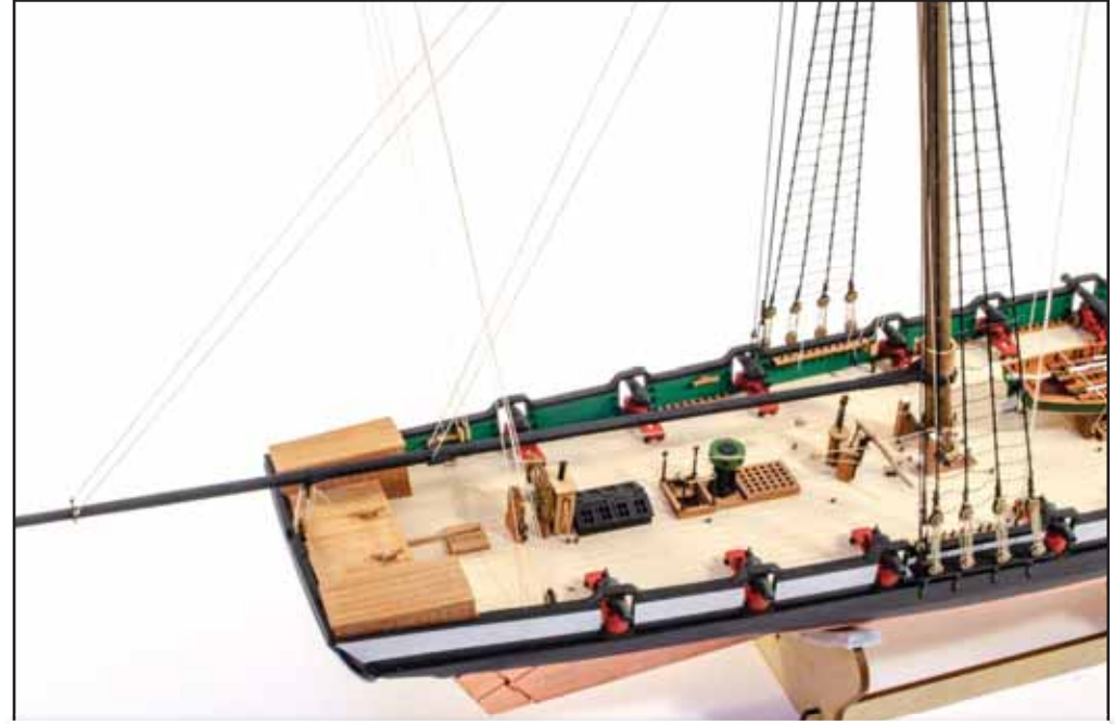
326. The gaff/boom assemblies can now be rigged. Ensure that all elevation and alignment of these parts is as close to the plans as you can get it before you seal any rope with glue. Here you see the main boom in situ.
