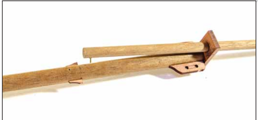
293. Here you can see this section about to be fitted. Note the hole drilled into the larger dowel, to accept the brass wire fitted in previous stage. Make sure all parts are properly glued too.
