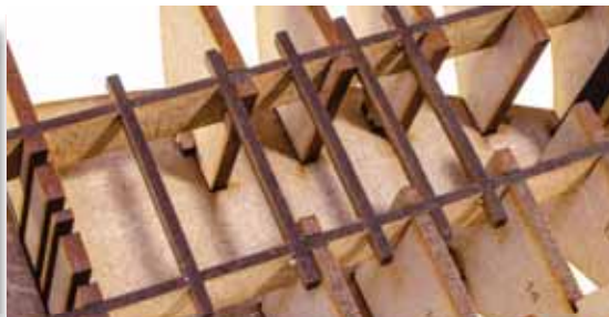
44. Glue across the specific slots in the top of the two longitudinal parts #29.
