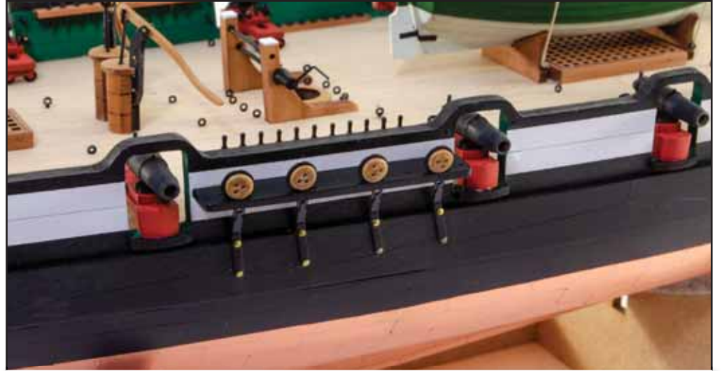
286. Using your plan as a guide to the angle/rake of the chainplates, fit the assemblies through the slots in the channels and glue/pin the chainplates to the side of the hull. Paint the brass pins in black. Here is the main mast channel...
