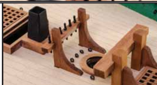
219. Assemble as shown and glue into position on the deck. When dry, add the same belaying pins as you did to the bulwark racks.
