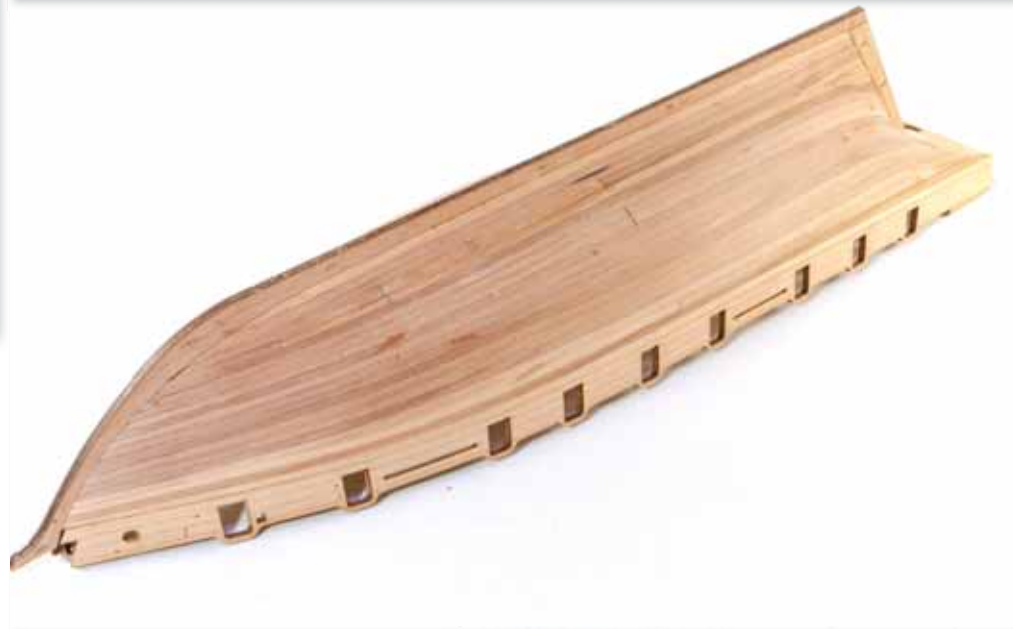
111. If you add any planks as halves, just do this if the need requires it. I have done this with a small number on either side. Here is the hull, completely planked.
