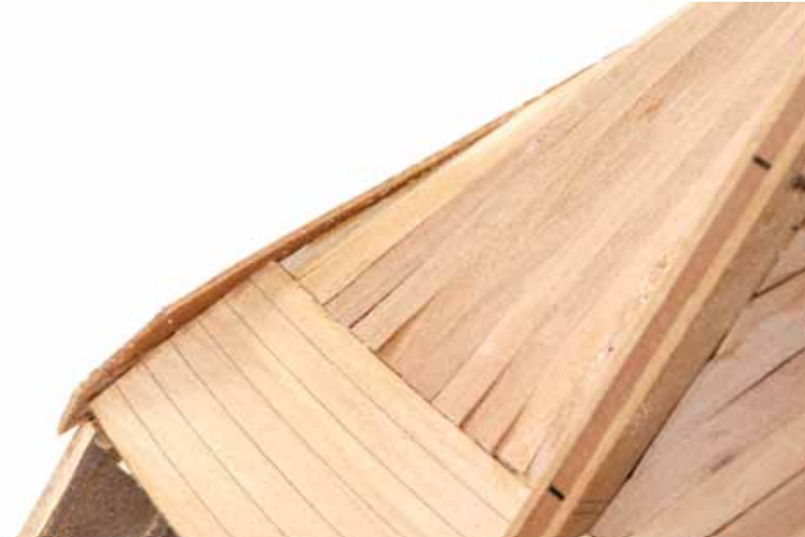
110. Now plank the hull again, using the pear wood strips, in the same manner as before. This photo shows you how the planks terminate at the part you just added, and also how they will look when they transition from the sides to the underside.
