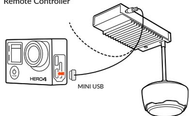
**STEP 1.** Plug the MINI USB connector into USB interface of GoPro Camera
