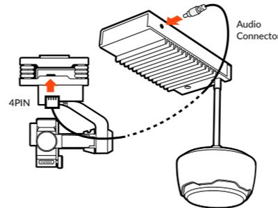
**IMPORTANT NOTE:** In this User Manual, the TYPHOON is taken as an example. If you have any other compatible power supply equipment or wearable equipment, you can plug the 4PIN power connector of the MK58 into power output port of other equipment as well.
