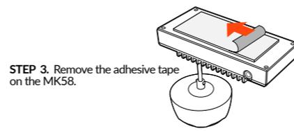
**STEP 3.** Remove the adhesive tape on the MK58.
