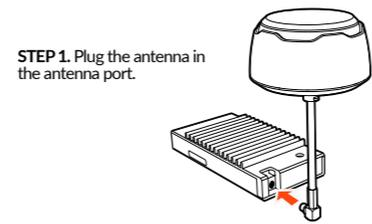
**STEP 1.** Plug the antenna in the antenna port.
