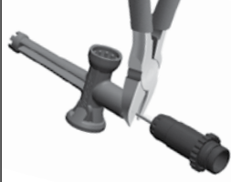
C. Remove/Install Rod End
