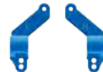
Aluminum axle carriers installed as labeled: 4° toe-in
