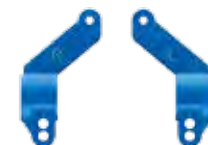
Aluminum axle carriers reversed: 1° toe-in
