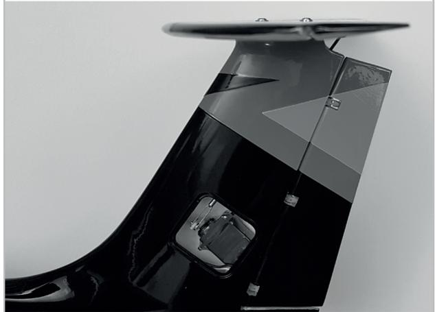
Check the length of the elevator linkage and, if needed, adjust it by adjusting the length of the clevis rods. The rudder should be placed in neutral position during a 90° position of the servohorn.
