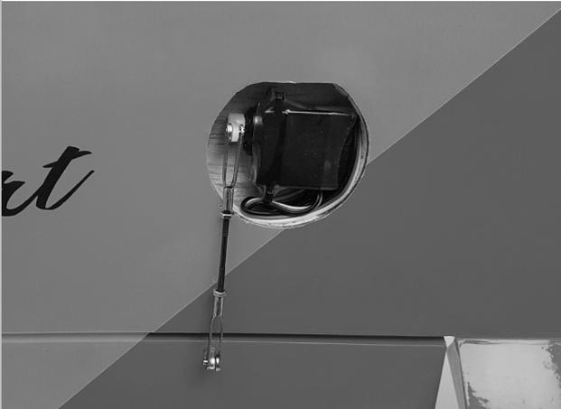
Connect the aileron rods to the rudder- and servo horns (outer servo). Make sure that the rudder is placed in neutral position during right-angled position of the servohorn. If needed, adjust the rods.
