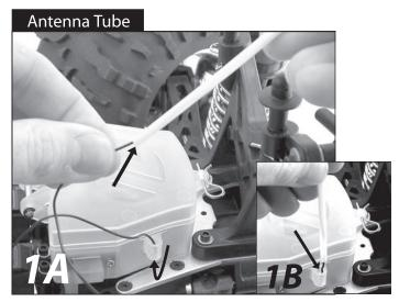
Find the antenna tube in the plastic bag with the Operations guide. Thread the black antenna wire attached to the receiver through the mounting boss (fig. 1A) on the right side of the radio box and through the antenna tube. Push the antenna tube (fig. 1B) into the mounting boss on the side of the radio box.
