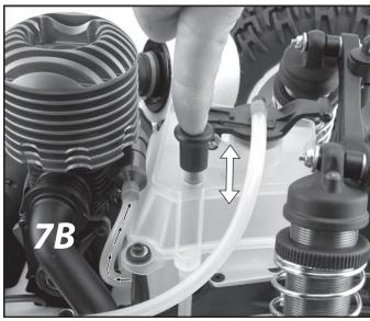
After filling the fuel bottle with fuel, lift the lid of the fuel tank and fill the tank (fig. 7A). Make sure you put the lid back on both the fuel bottle and the jug of fuel. Press down on the primer button several times (fig.7B) until you see the fuel move through the fuel line to the carburetor. Do not pump the primer after the fuel reaches the carburetor or you will flood the engine and make it difficult to start.
