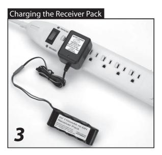
Plug the AC charger into the proper wall receptacle (110V). Plug the battery pack into the charger. When the battery is charging the red indicator light will be on. The battery must be charged for 12 hours to attain a full charge.
