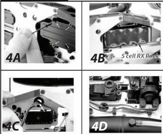
Note: Your LST2 is equiped with a rechargeable receiver pack installed in your truck. If needed, follow the instructions to remove or replace the
