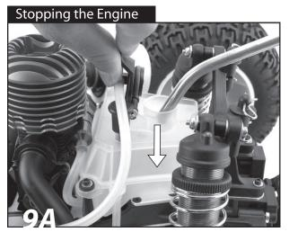
When you are done running your LST, push the primer button down to stop the engine (fig.9A). It may be necessary to push the primer button down several times. If the engine does not stop, use the handle of a screw driver or a rag to cover the exhaust pipe exit (fig.9B), being EXTREMELY careful not to burn your hand as this will be hot.
