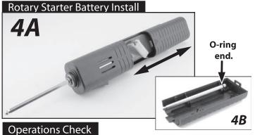
Slide the battery access panel opposite the hand strap back and remove the cover. Remove hex starter shaft from the back side of the cover (fig. 4b) and press the o-ringed end into the drive cup. Slide a 7.2 volt 6cell "stick pack" into the Spin-Start and plug it in. Note that the plug is made such that it can only be plugged in one way. Carefully tuck the plug wires under the battery access panel and slide shut.
