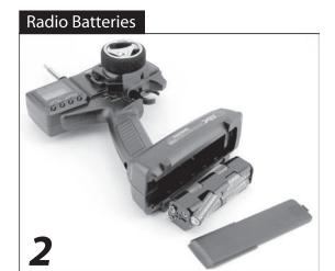
Install the 8 AA-size alkaline batteries in the transmitter making sure the positive (+) and (-) negative ends are oriented correctly. Use only quality alkaline or rechargeable Ni-Cad AA size cells.
