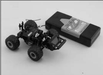
3. Plug the battery lead into the charger lead. The RED LED will light up and stay solid while charging. When the battery is fully charged the light will shut off (approximately 20 minutes). If the charger light only lights up for about a minute, the AA batteries inside the charger are low and should be replaced.
