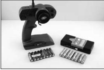
1. Your Losi Micro Raminator includes 2 complete sets of batteries. The Heavy Duty non-alkaline batteries are to be used in the transmitter.
