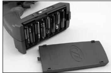
4. Remove the transmitter battery cover by sliding it in the direction noted on the cover. Install eight (8) AA batteries into the battery holder. Pay close attention to the correct direction of the positive (+) and negative (-) ends as marked. Once all 8 batteries have been installed, reinstall the battery cover.
