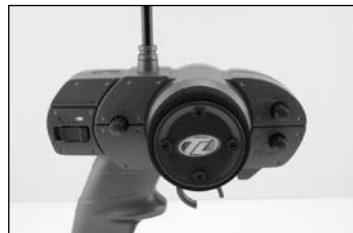
6. ALWAYS turn on the transmitter first by sliding the switch "ON". The small red and green lights above the switch should both light up. If not, please check for low or incorrectly installed batteries.
