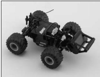
5. Plug in the battery lead into the speed controller lead and replace the body. Secure the body with the included body clips.
