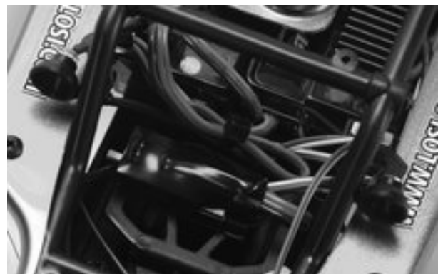
Plug the lead from the light module into the AUX port on the Receiver. Using double-sided tape (included), mount the LED Light Module in front of the ESC and Receiver on the battery hold down.
