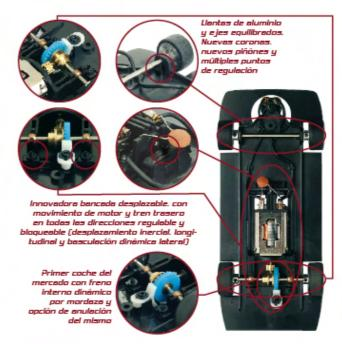
bronze for greater toughness. You can experiment with the different gearings which are possible with these **SCX® PRO** models.
