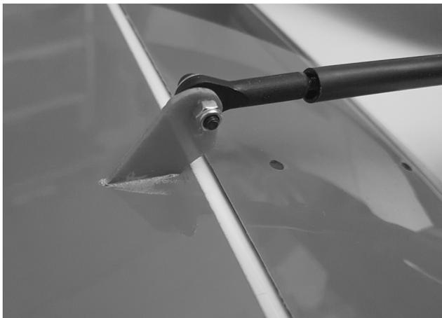
Screw the M3 ball stud into the outer bore of the rudder horn.
