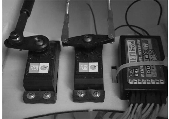
Now, the rudder servo arm can also be plugged in 90 ° position on the servo in neutral position. Pay attention to a certain bias of the ropes.
