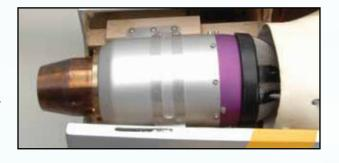
Epoxy the turbine mounting blocks into place, ensuring that they do not move whilst the epoxy is curing.
