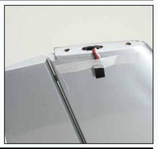
Install the rudder servos as shown, with the output arm towards the front of the boom. Attach the control horn to the rudder and make up the rudder pushrod in the same way as per the elevator connection previously making sure that keepers are fitted to the clevises for security. Repeat for the second tail boom.
