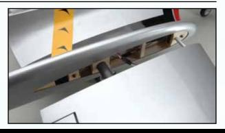
The wing panels are retained using the pre-installed moulded clamps onto the wing joiner ends.
