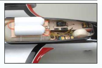
More installation detail showing ECU and I/O board, as well as the retract and brake air valves and servos. Note the small screw at the rear of the left side equipment tray, this retains the rear end of the tray whilst the front end locks into the former at the front of the equipment bay. The right side equipment tray is secured in a similar manner.
