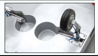
Check that the legs/wheels retract fully, a small amount of trimming of the underside fuselage skin may be required to achieve this.
