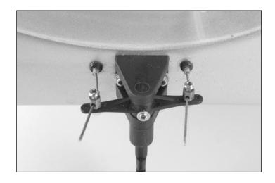
Rudder linkage setup.
