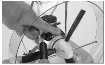
O 2. To prime your engine, first turn on your transmitter and then your receiver. Move the throttle to full open and place your finger over the carburetor opening. Turn the propeller over by hand until you can see fuel entering the fuel line. Move the throttle stick full down to idle.
