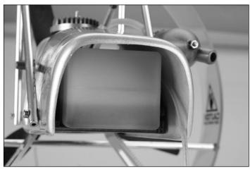
Checking the fuel level from rear of engine pod.
