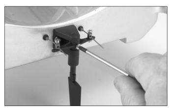
3. Find the predrilled hole in the rudder shaft. Using a #1 Phillips screwdriver, tighten the screw as shown.
