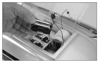
3. Remove the dry cell battery holder from the radio box and unwrap the foam from around the dry cell battery holder. Install 4 "AA" alkaline batteries as shown. Note the proper polarity. Wrap the battery box in foam.
