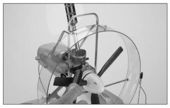
○ 3. Move the throttle to the low position and the throttle trim lever to the middle position. Place the glow driver on the glow plug and, using a start stick, turn the propeller counter clockwise through the compression stroke. You should feel a "bump" against the start stick. When you feel the "bump", flip the propeller counter clockwise to start the engine. Repeat the process if the engine does not start.
