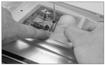
4. Re-install the battery holder into the radio box and properly seal the radio box with clear tape. Failure to properly seal the radio box could result in damage to your radio equipment. Insert the receiver antenna tube into the clear lid.
