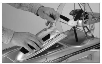
O I. Remove the knurled aluminum nut that secures the cockpit. Pull the cockpit off the boat.
