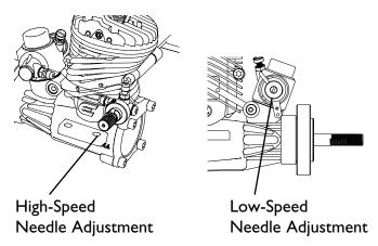
**Warning**: Make all adjustments to the Evolution engine's low-speed needle valve with the engine stopped.
