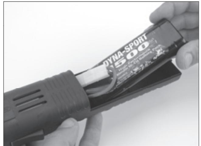
1. Fully charge a 7.2V sub-C battery pack and install it in the starter as shown.
