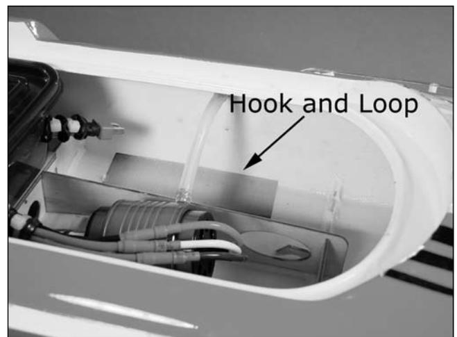
Confirm that the switch inside the boat is in the "OFF" position. Install two fully charged 7.2V Ni-MH battery packs into the hull.
