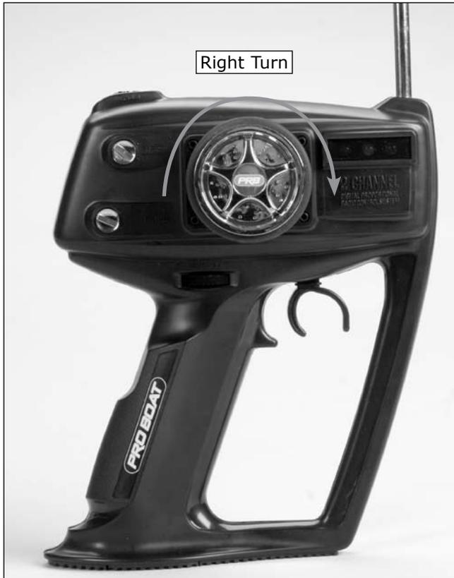
The ESC will beep until you give full throttle input. The auto sensing circuitry will select full throttle position when you hold full throttle during initial setup. Release the throttle trigger. With the propeller free from any objects, give some throttle input to ensure that the motor is working. If everything appears to be functioning correctly, you are ready to run your boat.
