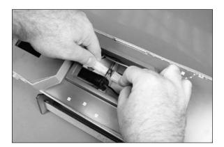
O 7. Check the operation of the rudders in relationship to the steering wheel. When the wheel is rotated clockwise, the rudders must move right as shown. If not, follow the instructions from the radio to set the servo reversing for the steering.
