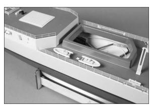
O 5. Accessory item E and location. Use a pin vise and 5/64-inch (2mm) drill bit to enlarge the hole in the hull for the accessory as shown before installation.
