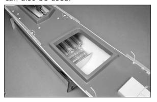
O 5. Place the motor battery in the hull. The supports are cut to fit a 6-cell battery snug in the hull.
