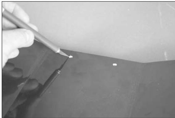
□ 3. Use 30-minute epoxy to glue the two 6mm x 30mm dowels in the leading edge of the wing. Make sure the dowels are positioned so 3/8-inch (10mm) of the dowel is exposed forward of the leading edge as shown.
