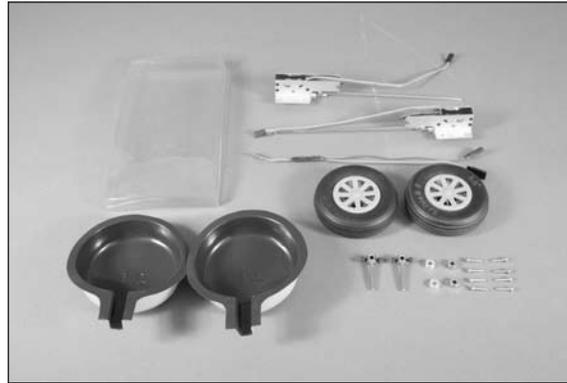
□□ 2. Use the radio system to extend the retracts to the open position. Use a rotary tool and cutoff wheel to trim the retract strut length to 4⅛ inches (105mm) from the top of the wheel collar. Use a flat file to remove any burrs after trimming the strut length.
