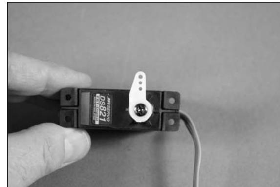
□□ 5. Place the servo on the cover, centering the servo horn in the opening. Use a pencil to mark the locations for the servo mounting blocks on the servo cover.
