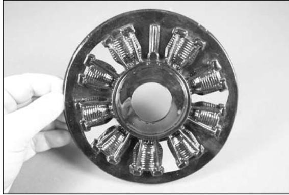
□ 4. Fit the dummy engine over the engine. Trim the dummy engine as necessary so the drive washer is exposed forward of the dummy engine.
