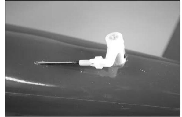
**Note:** The arm on the adapter will angle toward the rear of the fuselage. This is necessary so the pushrod does not bind when operating the rudder.
