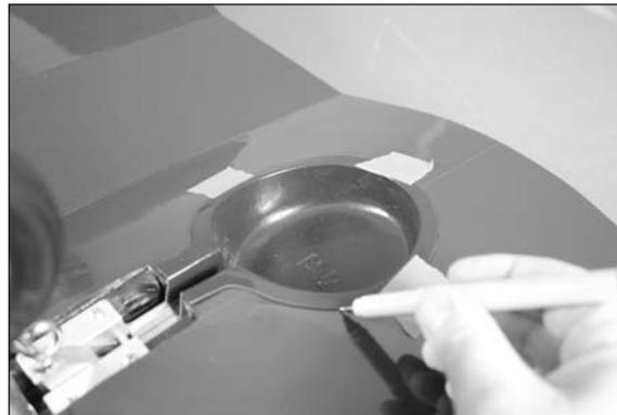
□□ 31. Use a hobby knife with a new #11 blade to remove the covering 5/64-inch (2mm) inside the line so the wheel well can be glued to the exposed wood.
