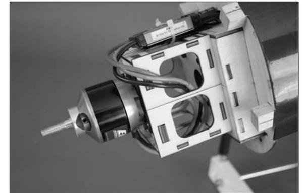
**Note:** If you are installing an E-flite motor and speed control, you can match the colors from the motor and ESC. This will result in the motor rotating the correct direction for your model.
