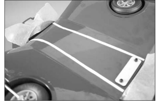
**Note:** Make sure to use a new #11 blade and use light pressure to trim only the covering. Avoid cutting into the underlying wood, which could weaken the structure of your model.
