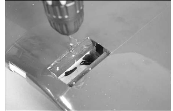
□□ 9. Use a #2 Phillips screwdriver to thread a #4 x 3/4-inch sheet metal screw into each of the four holes drilled in the previous step. This will cut threads into the surrounding wood. Remove the screw before proceeding to the next step.
