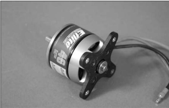
□ 11. Attach the propeller adapter on the motor using the hardware provided with the adapter.
