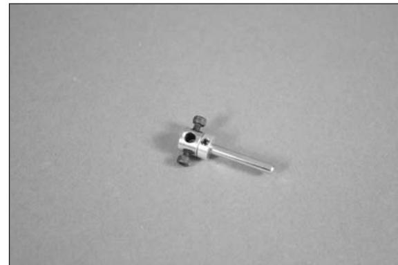
□□ 20. Remove the hub cap from the main wheel. Slide the wheel on the axle with the side opposite the hub cap facing the wheel collar.
