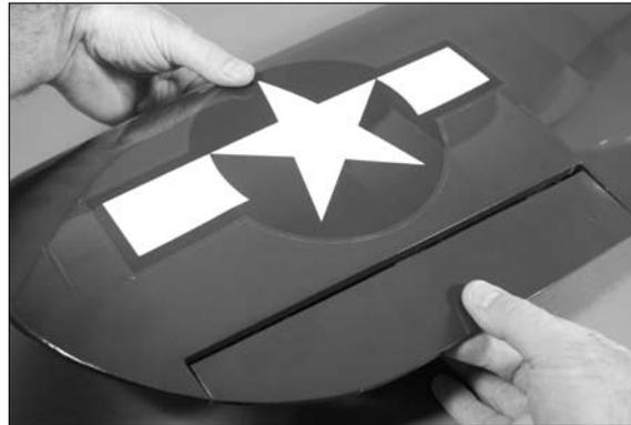
□□ 7. Break in the hinges by working the aileron up and down a number of times.
