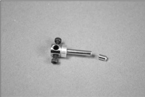
□□ 23. Use a flat file to make a 1/4-inch (6mm) wide flat at the end of the axle.
