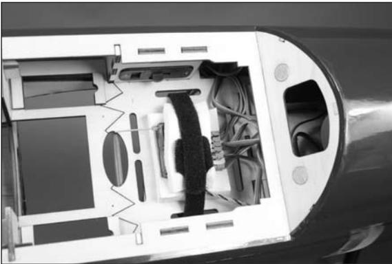
□ 17. Mount the remote receiver in the airframe using hook and loop tape. Make sure the antenna on the remote receiver are 90-degrees in relationship to the main receiver antenna. Place the remote receiver as far away from the main receiver as possible for the best radio reception.
