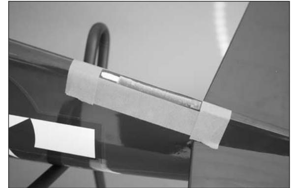
□ 17. Apply a thin coat of petroleum jelly to the torque rod to prevent accidentally gluing the rod into the bushing if epoxy happens to run down into the fuselage.
