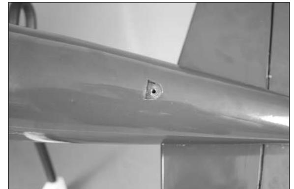
□ 12. Test fit the rudder assembly into the fuselage. Make sure to slide the torque rod into the tube inside the fuselage. Check that the bottom edge of the balsa fairing rests flat on the fuselage. The fin will also rest tightly against the top of the fuselage. If not, remove the covering from the bottom of the fin or even lightly sand the bottom of the fin where it contacts the fuselage to correctly position the balsa fairing.
