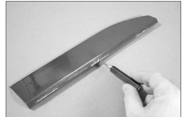
□□ 3. Place a T-pin in the center of three hinges. Insert the hinges into the aileron as shown. The hinges have a slot in them and must be installed so the slot is perpendicular to the hinge line of the control surface.
