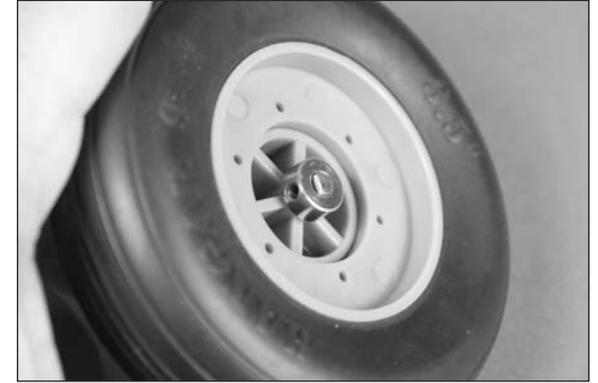
**Note:** If you choose to use a 1.5mm ball driver to tighten the setscrew make a small notch in the wheel hub to reduce the angle of the hex wrench so it fits the setscrew better and to reduce the chance of stripping the setscrew.
