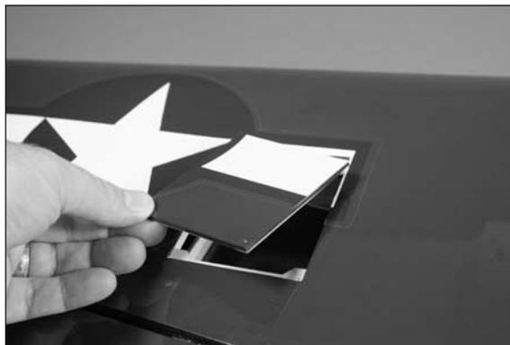
□□ 3. Use a hobby knife with a #11 blade to remove the covering for the servo horn to pass through the servo cover.
