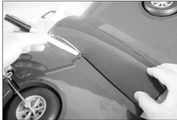
**Hint:** The fiberglass belly pan may not lay flat against the wing. Use a washcloth soaked in hot water to warm the fiberglass, making it pliable so you can mold it to the wing contour.
