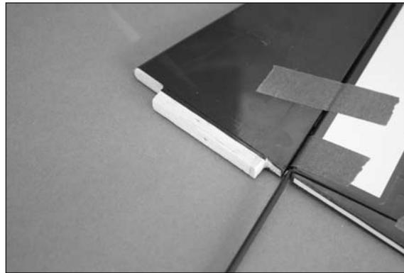
**Note:** Make sure to use a new #11 blade and use light pressure to trim only the covering. Avoid cutting into the underlying wood, which could weaken the structure of your model.
