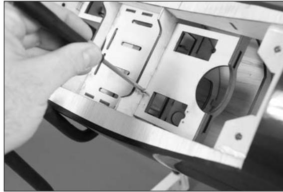
□□ 6. Apply 2–3 drops of thin CA in each hole drilled. This will harden the surrounding wood, making the screws more secure when installed.
