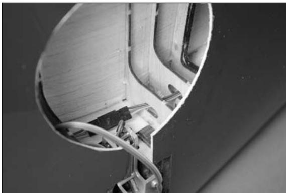
□□ 18. Check the fit of the wheel well into the wing. You may need to use a rotary tool and sanding drum to adjust the opening to allow the well to fit. It may also be necessary to notch the wheel well to clear the top of the retract chassis. Use low-tack tape to hold the wheel well in position. Do not glue the wheel well at this time.
