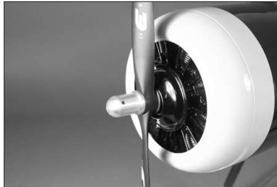
**Note:** It may be necessary to use a reamer to enlarge the hole in the propeller to fit the motor shaft. Always balance your propeller. An unbalanced propeller can cause vibrations to be transmitted into the airframe, which could damage the airframe or other components as well as produce unwanted flight characteristics.
