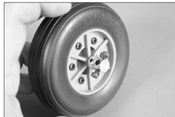
□□ 21. Slide the wheel collar from the kit (this collar has a chrome finish) onto the axle. With the axle pressed against the backside of the wheel, use a felt-tipped pen to mark the axle at the edge of the wheel collar.
