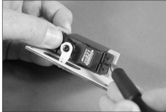
□□ 9. Use a drill and 1/16-inch (1.5mm) drill bit to drill the holes for the four mounting screws.
