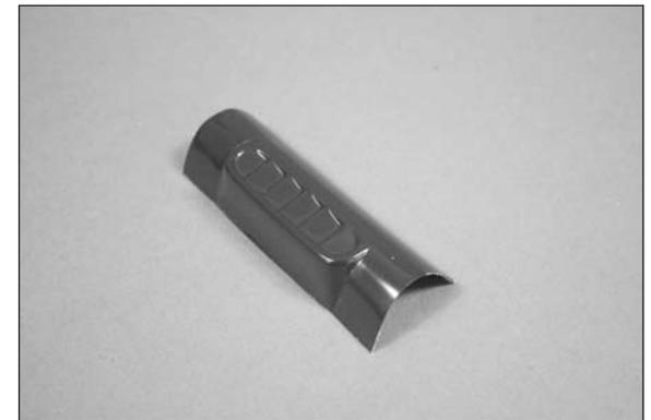
**Hint:** Radius the corners to minimize catching an edge when you wipe the model down with a towel.
