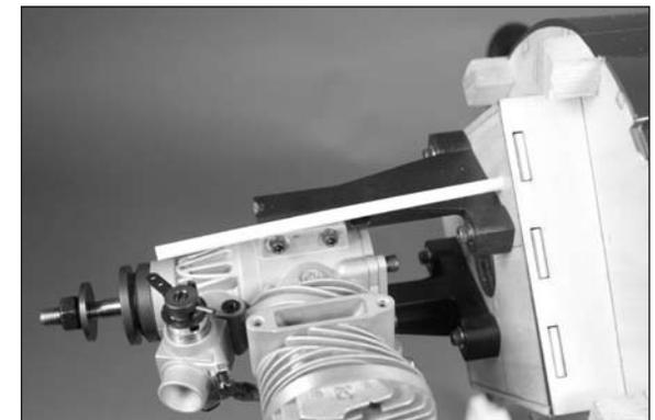
□ 10. Use side cutters to trim the tube flush to the rear of the engine mounting lug.
