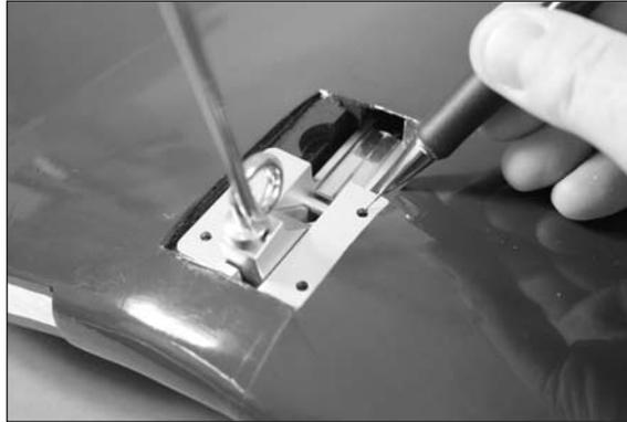
□□ 7. Place a 5/64-inch (2mm) drill bit in the drill. Wrap a piece of tape around the drill bit 3/4-inch (19mm) from the end of the drill bit to prevent accidentally drilling through the top of the wing.
