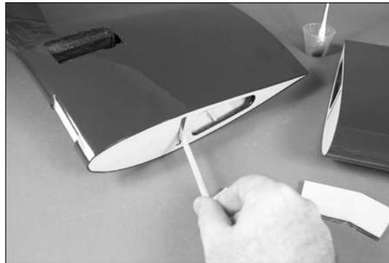
□ 8. Use an epoxy brush to apply epoxy to all sides of the wing joiner. It is important the joiners have epoxy at all points where they come in contact with each other.
