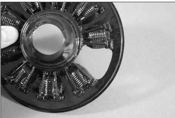
□ 3B. (EP Only) Remove the material between four of the cylinders to allow cooling air to pass over the motor and speed control.
