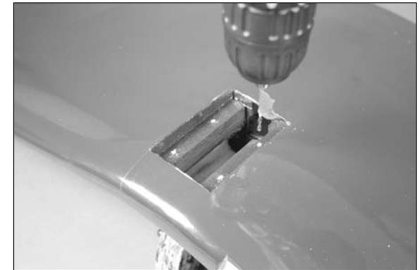
□□ 8. Use a #2 Phillips screwdriver to thread a 3mm x 15mm black counter sunk screw into each of the four holes drilled in the previous step. This will cut threads into the surrounding wood. Remove the screw before proceeding to the next step.
