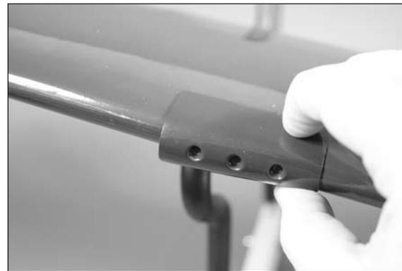
□□ 7. Use a drill and 1/4-inch (6mm) drill bit to drill the remaining two locations so the machine gun can rest tightly against the leading edge of the wing.
