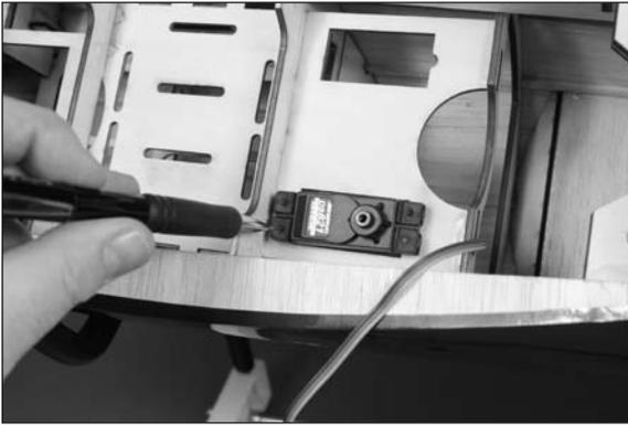
□□ 4. Use a pin vise and 1/16-inch (1.5mm) drill bit to drill the holes for the four mounting screws.
