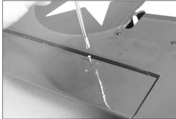
□□ 7. Apply 2–3 drops of thin CA in each of the holes that will accept the servo cover mounting screws.
