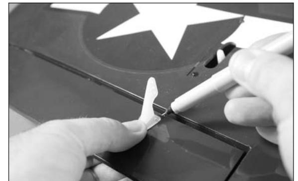
□□ 4. Place a 1/16-inch (1.5mm) drill bit in the drill. Wrap a piece of tape around the drill bit 5/16-inch (8mm) from the end of the drill bit to prevent accidentally drilling through the top of the aileron.
