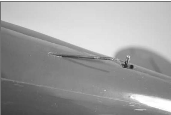
□ 11. Repeat steps 3 through 9 to install the elevator servo and the 2mm x 610mm elevator pushrod in the fuselage.
