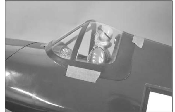
□ 10. Measure back 2½-inches (63mm) and use a hobby knife with a #11 blade to cut a small opening for the antenna mast. Start small and work up until the mast just fits into the opening.
