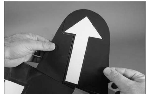
30. Break in the hinges by moving the rudder through its range of throw a number of times.
