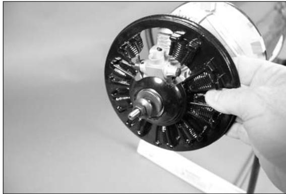
**Note:** It may be necessary to increase the amount of inlet area around the cylinders as needed for each of the engine applications. Too much inlet air will cause pressure inside the cowl and actually cause more heating issues. The goal is to have adequate outlets in the cowling to allow the incoming air to escape.
