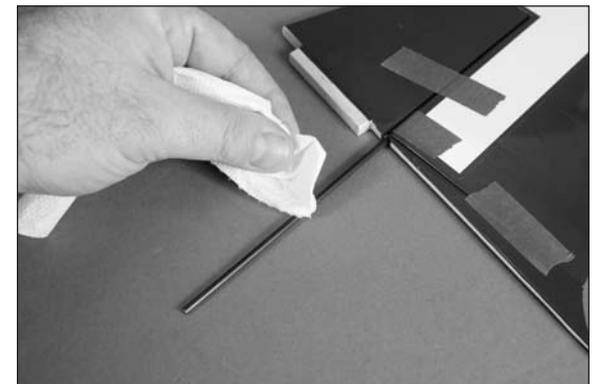
**Important:** Make sure to use enough epoxy to glue the fin securely to the fuselage. Not using enough epoxy may result in a poor bond between the fin and fuselage, which could cause the fin to loosen in flight.
