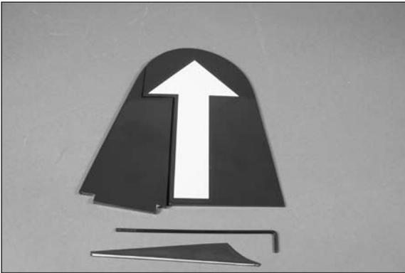
□ 2. Separate the rudder from the fin. Set the fin and two CA hinges aside.
