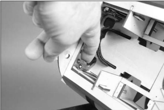
□ 17. The battery is secured in the fuselage using the hook and loop strap. We also recommend using a piece of hook and loop tape between the battery and battery tray to keep the battery from accidentally moving inside the fuselage.
