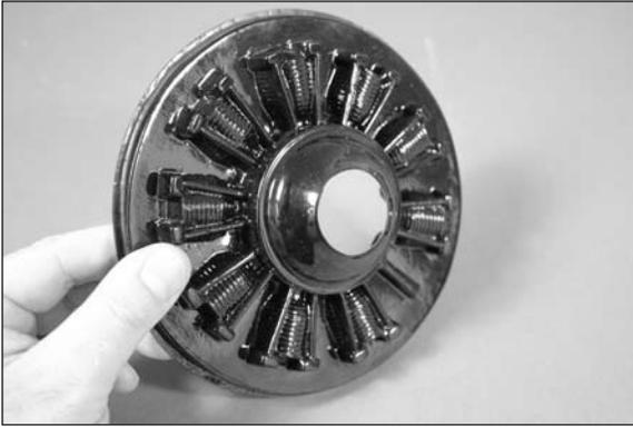
□ 3A. (Glow/Gas Only) Remove the area between the cylinders as shown to clear the carburetor on the engine. Choose the section that has the widest gap between cylinders. This will allow you to see the carburetor to position the dummy engine in the cowl. This hole will be enlarged in the following step.
