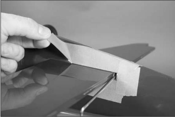
□ 18. Once the epoxy fully cures, the wing can be removed from the fuselage by removing the two 8-32 bolts using a 9/64-inch hex wrench.
