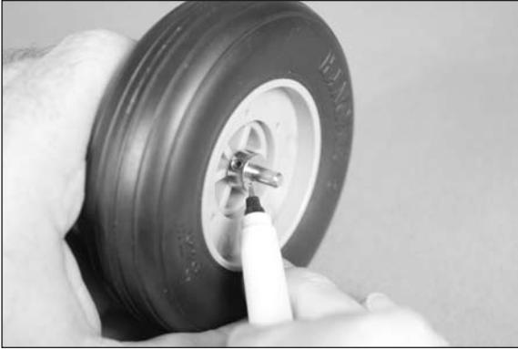
□□ 22. Remove the wheel and wheel collar from the axle. Use a rotary tool and cutoff wheel to trim the length of the axle at the mark made in the previous step. Use a flat file to remove any burrs left from trimming the axle.
