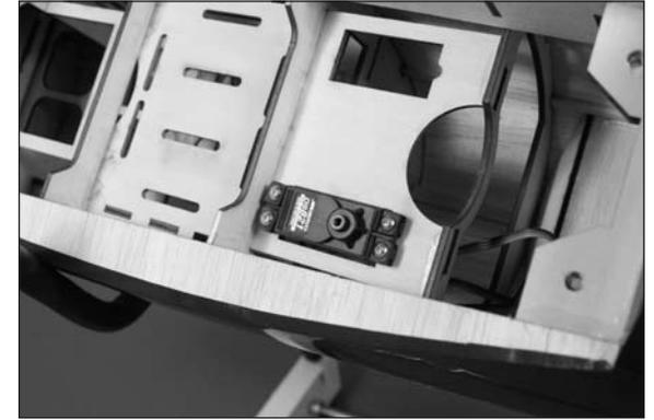
□□ 8. Use a pin vise and 5/64-inch (2mm) drill bit to enlarge the hole in the servo arm that is 1/2-inch (13mm) from the center of the arm. Use side cutters to remove any unused arms so they don't interfere with the operation of the servo.
