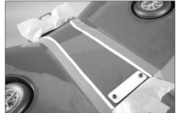
12. Mix 1/2 ounce (15mL) of 30-minute epoxy. Use an epoxy brush to coat the exposed wood on the bottom of the wing. You will want a nice build-up of epoxy to guarantee that it fully contacts the belly pan.
