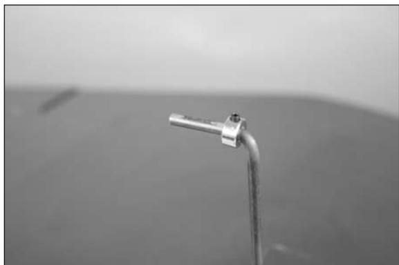
□□ 12. Place a drop of light machine oil on the axle.
