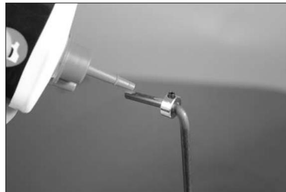
□□ 13. Remove the hub cap from the main wheel. Slide the wheel on the landing gear wire with the side of the wheel that had the hub cap toward the wing tip.
