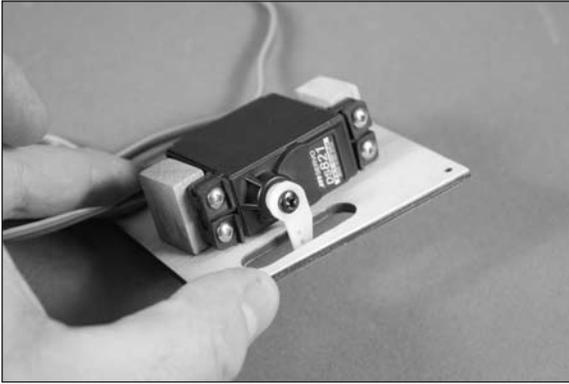
□□ 13. Secure a 12-inch (305mm) servo extension to the aileron servo lead using string or a commercially available connector. Use tape to temporarily attach the extension if you are installing the optional retracts.
