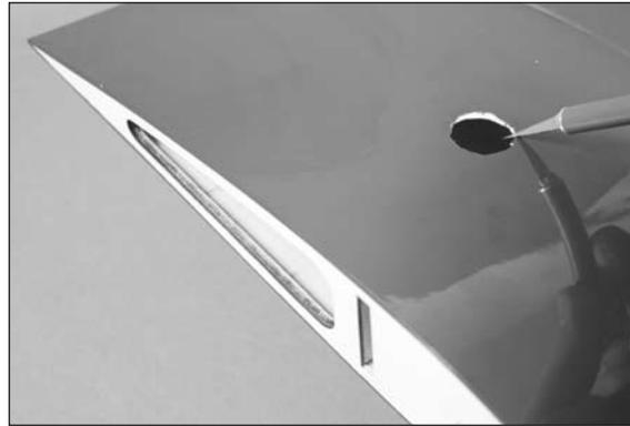
**Note:** It is important the joiner and joiner pockets have epoxy at all points where they come in contact with each other.
