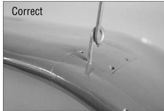
□□ 5. Use a pencil to transfer the locations for the mounting screws onto the landing gear rails inside the wing.
