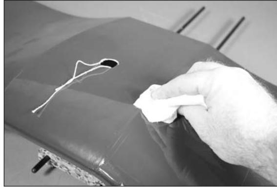
□ 12. Use a covering iron to apply the two strips of covering over the joint between the outer panels and the center panel starting at the trailing edge and wrapping the covering strip around the leading edge in one piece. This will eliminate any seams which could come loose in flight.
