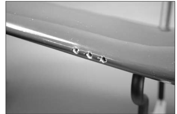
□□ 8. Test fit the machine gun to the wing. You may need to chamfer the holes with a hobby knife and #11 blade slightly to get the machine gun to fit tightly against the wing. Once satisfied with the fit, use canopy glue to secure the machine gun to the wing. Hold the machine gun in position using low-tack tape until the glue cures.
