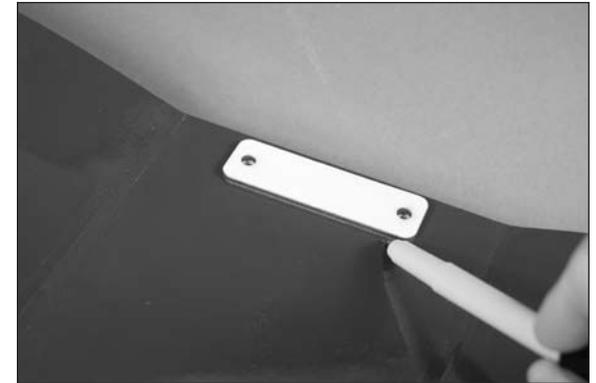
□ 5. Use a hobby knife and a #11 blade to trim the covering 1/16-inch (1.5mm) inside the line drawn on the previous step. Remove the covering from the bottom of the wing.
