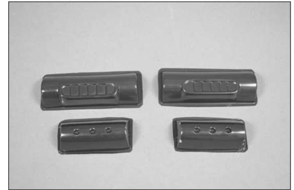
□□ 2. Use a hobby knife with a #11 blade and hobby scissors to remove the flashing from the radiator. Also remove the ends so the radiator can fit to the wing.
