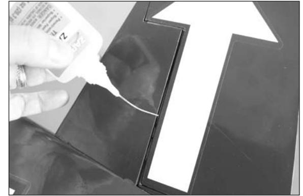
**Important:** Allow the CA to cure WITHOUT using CA accelerator. This is necessary to allow the CA to soak into the hinge, creating the best bond between the hinge and surrounding wood.
