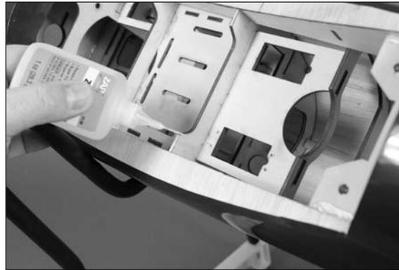
**Important:** Do not use a CA accelerator. Using an accelerator will not allow the CA to soak into the fibers of the wood, hardening the blocks.
