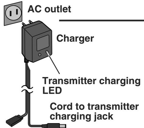
When charging the NT8F1100B NiCd battery with the special charger FBC-19B(4) (for U.S.A.), allow about 24 hours for charging. If the transmitter has not been used for some time, cycle the battery by charging and discharging it two or three times.
