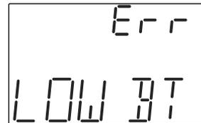
The low battery alarm is meant to be a safety feature only. Do NOT operate your radio below 9V. Always shut your radio off as soon as possible after the low battery warning tone to avoid loss of control.
