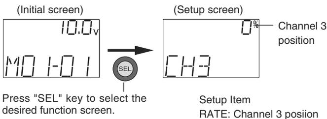
When channel 3 switch is operated, the "CH3" screen is displayed automatically for about three seconds.
