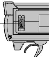
Note: Always set the F/S position when turning on the transmitter power.
