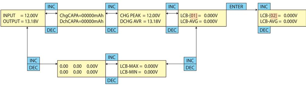
If the Battery TYPE button is pressed for over 3 seconds, the Data view will be displayed as above. Data displays can be scrolled left and right by using the INC & DEC buttons. If the Battery TYPE button is pressed again, the data view screen will disappear.
