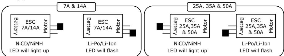
The jumper plug is fitted to the Airpower 7A & 14A plug onto the opposite end of the speed controller than the 25A, 35A and 50A so pay particular attention that the jumper plug is positioned correctly for your speed controller.
