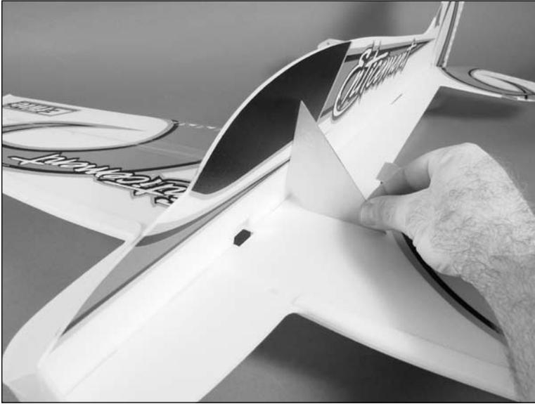
**Note:** Use low-tack tape to tape the control surfaces in their neutral positions. This will make the airframe easier to handle during assembly. Be careful not to tape the printed surfaces as there is a chance of the printing coming off when removing the tape.
