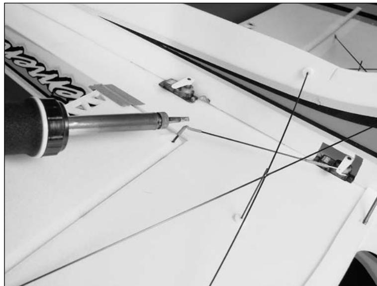
**Note:** You must use a soldering iron to shrink the tubing. The heat from other methods cannot be controlled as well and will cause damage to your airframe.
