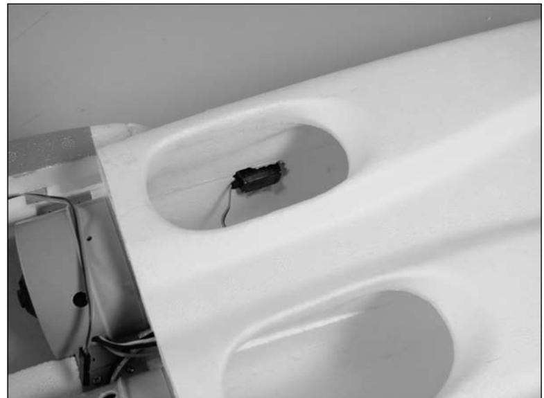
**Note:** Some early kits may need to have the retract units changed for this application. Please check your retract units with the pictures. The actuation arm should exit the same side as the gear strut wire when retracted. If so, skip to Step 8 on the following page of this manual.
