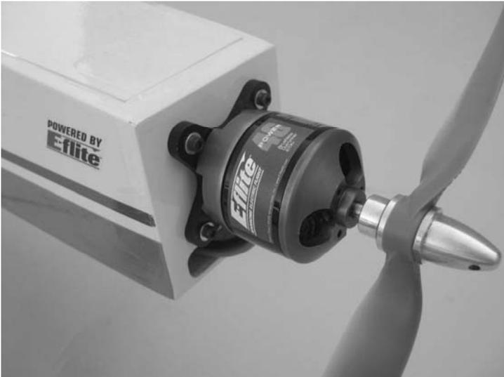
**NOTE:** Photo shows typical installation of motor and x-mount directly to the outside of the firewall. There are other options available including mounting the motor inside the fuselage (requires reversing the shaft direction) or extending the motor further forward using aftermarket mount extensions when using cowls.
