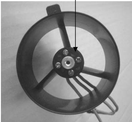
Screw Attaching Rotor
