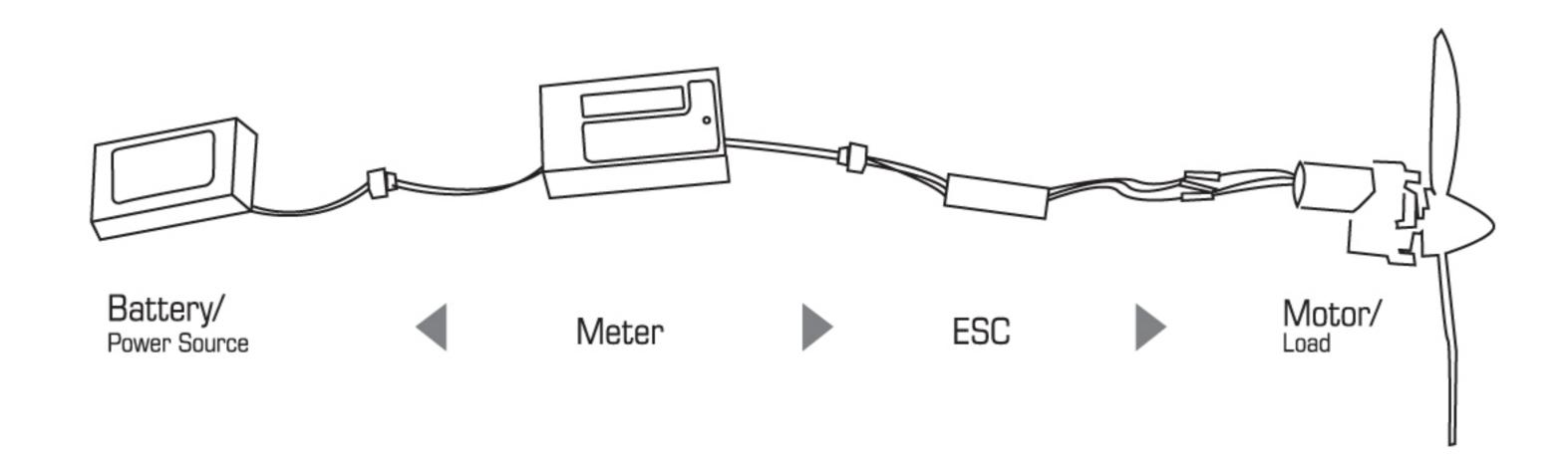
The Power Meter is designed to use in-line. It displays Volts (V), Amps (A), Watts (W) and Capacity (mAh) based on your MODE selection. Connectors are not included, allowing you to customize the meter to fit your needs. When soldering connectors onto the lead wires, be sure to use heat shrink tubing to properly insulate the wires so they will not short. Shorting may damage the meter.
