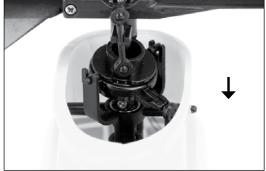
With the stick pushed right, the left-hand servo should push the swashplate upward.
