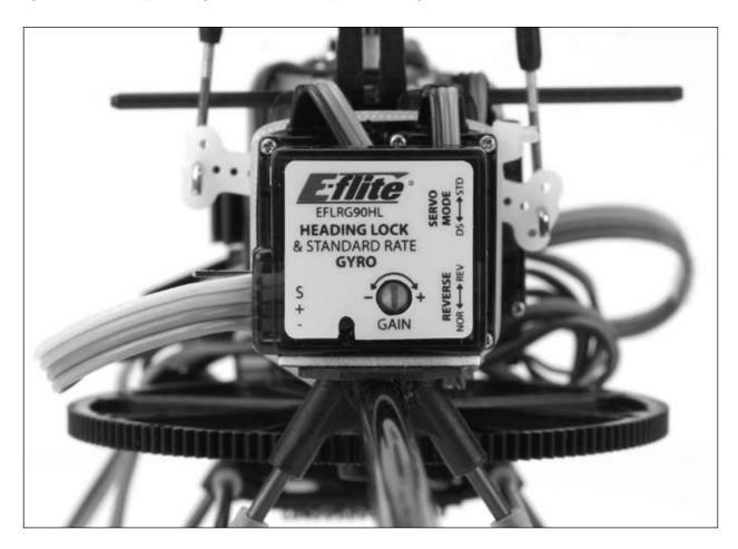
• If you are using the G90 gyro, and have chosen to utilize the remote mode and gain setting control option, you will need to use the Channel 5 knob on the transmitter for setting the mode type and gain value, as outlined in the following steps:
