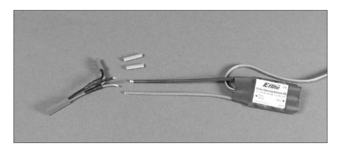
• Once the Y-harness has been connected to the ESC's battery power leads, and the joints have been properly insulated, you can now proceed with installation of the ESC on the helicopter. There are a few places in which the ESC can be mounted on the helicopter, including the following:
