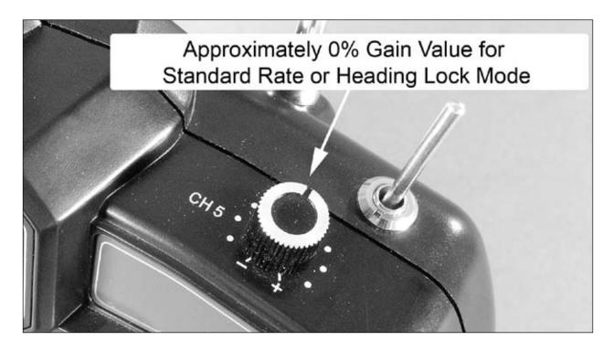
When the Channel 5 knob is rotated counterclockwise (-) from the middle position, the gyro will be in the Standard Rate mode. This mode is the same as offered by the 3-in-1 control unit's stock gyro. When the knob is rotated full counterclockwise, the gain setting value will be approximately 100%. Other gain setting values from approximately 0–100% are also available depending on where the knob is set between the middle and full counterclockwise positions.
