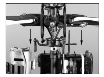
With the stick pulled back down, the swashplate should raise, decreasing the pitch of the main blades.
