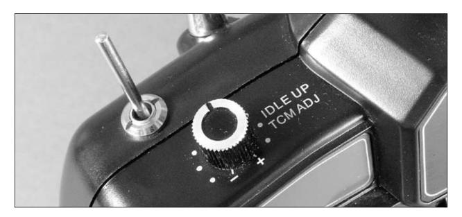
When the knob is in the highest, most clockwise position (+), the midpoint of the throttle curve in the Idle Up/Stunt flight mode will be approximately 100%.
