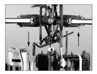
With the stick pulled back, the swashplate will tilt toward the rear.
