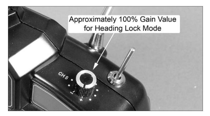
We recommend that you set the Channel 5 knob in the position that provides a gain setting value of approximately 50% in the Heading Lock mode before conducting the first test flight after installing the gyro. You will then use the Channel 5 knob on the transmitter for adjusting the gyro gain value after conducting test flights.
