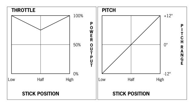
With the Idle Up TCM ADJ knob in the highest, most clockwise position.
