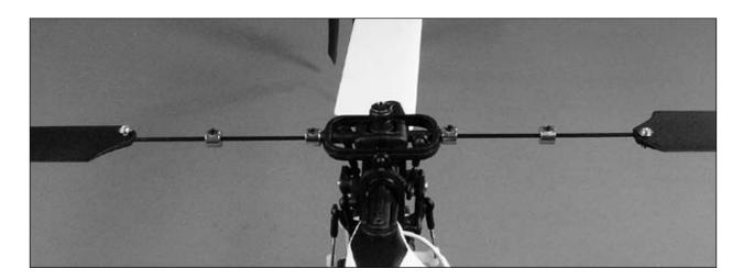
Dampening of the rotor head (main rotor blades) can also be adjusted in order to fine-tune the cyclic response of your model. In general, stiffer dampening will result in quicker cyclic response. The dampening of your Blade™ CP Pro has been set to provide a good balance of cyclic response and stability right out of the box, and we suggest that you make your first flights with this amount of dampening before making any changes.
