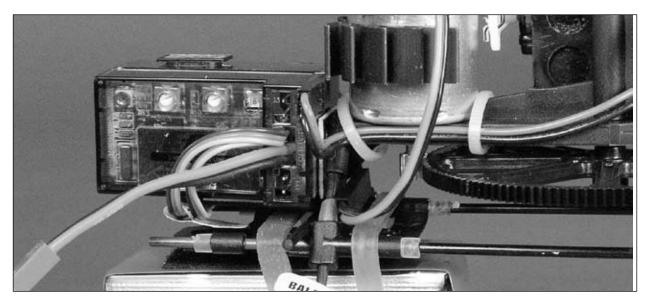
Turn the transmitter on first and lower the throttle stick and trim completely. Then, plug the battery into the battery lead of the 3-in-1 unit.
