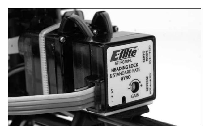
• Remove the 3-in-1 control unit's rudder channel lead (marked with a small label) from channel 4 of the receiver, and plug this lead into the servo connector of the gyro. Then, plug the rudder channel lead of the gyro into channel 4 of the receiver, ensuring proper orientation and polarity direction of the wire leads.
