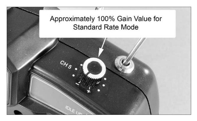
When the Channel 5 knob is rotated clockwise (+) from the middle position, the gyro will be in the Heading Lock mode. This is the mode that is preferred for use after installing the heading lock type gyro. When the knob is rotated full clockwise, the gain setting value will be approximately 100%. Other gain setting values from approximately 0–100% are also available depending on where the knob is set between the middle and full clockwise positions.
