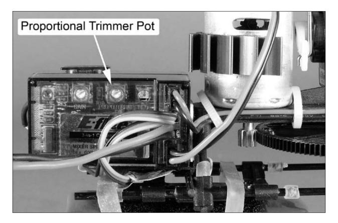
• In hover, with the rudder trim centered and no rudder input, note which direction the nose of the helicopter is trying to spin. If the nose of the helicopter is spinning to the left, you will want to increase the amount of tail motor to main motor mixing. By turning the proportional trimmer pot clockwise (+), you increase the tail motor/rotor rpm for a given main motor/rotor rpm. This increase in tail motor/rotor rpm will help to push the nose of the helicopter to the right when in hover.
