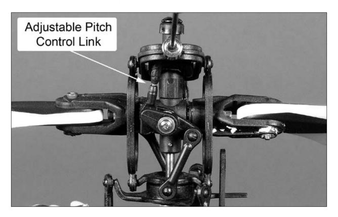
In general, we would recommend that you adjust the Pitch Control Links so that the blades are at 0 degrees of pitch when in the Idle Up/Stunt flight mode with the throttle/collective stick in the middle position. This will help to ensure that you have an equal amount of positive and negative pitch travel when in the Idle Up/Stunt flight mode, and that your curves more closely match those shown in the "Programmed Throttle and Pitch Curves" sections of this manual (pages 31–32).
