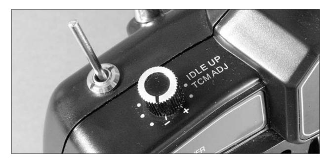
When the knob is in the middle position, pointing directly toward the back of the transmitter, the midpoint of the throttle curve in the Idle Up/Stunt flight mode will be approximately 75%.
