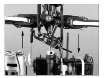
While viewing the helicopter from the rear (tail boom toward you), move the right-hand stick left and right to check aileron roll control. When the stick is pushed to the left, the swashplate should also tilt left.
