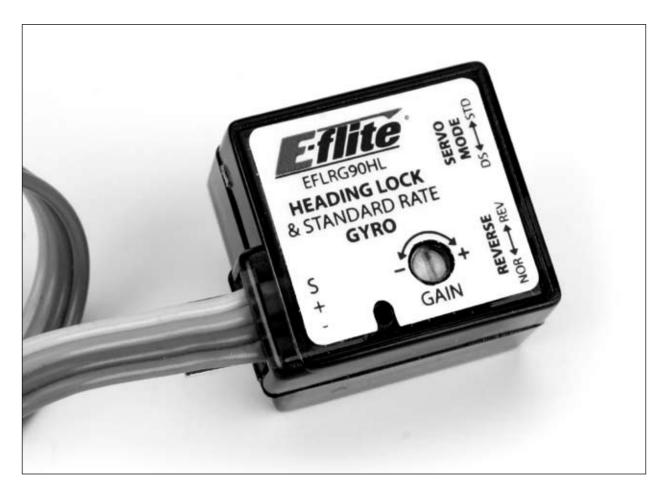
Note: The following steps outline the installation and setup of the G90 gyro, but can also be used as reference for many other heading lock type gyros. However, we do recommend that you review the manual included with your chosen gyro first before proceeding with installation and setup of the gyro in your Blade CP Pro.
