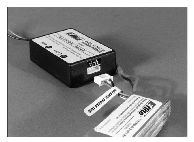
When the battery is properly connected and charging normally, the red and green LED indicators will glow solid. Once the battery has been fully charged, the green LED will go out, leaving just the red LED glowing solid. The battery can now be removed from the charger and installed on the Blade™ CP Pro for flight.
