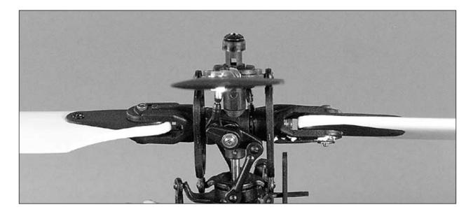
• Once you have positioned the flybar paddles correctly following the steps above, be certain they are firmly secured using the included screws, washers and hex nuts.
