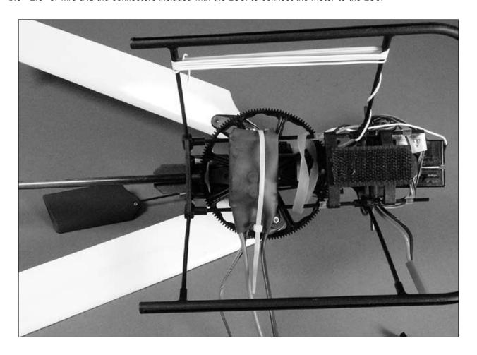
After securing the ESC in its mounting position, connect the motor wire leads to the connectors on the ESC.
