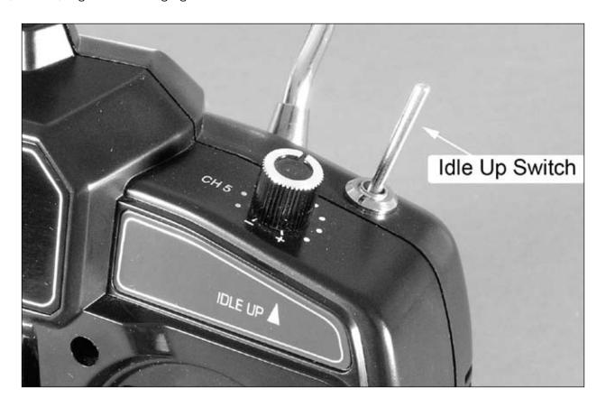
When the "Idle Up" switch is toggled toward the rear of the transmitter, the Blade<sup>TM</sup> CP Pro will be flying in "Normal Mode." In this flight mode, the throttle curve is linear from 0% to 100%, with a pitch range of approximately -1 degree to +12 degrees. (See page 31 for additional data and graphics relating to the throttle and pitch curves preset for your Blade CP Pro.) This is the preferred flight mode for general hovering and gentle forward flight.
