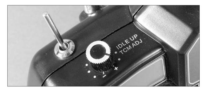
The unique benefit of this knob is that it offers you the ability to adjust the main rotor head speed, and in turn the collective and cyclic control response, of the model between the endpoints of the throttle curve when in the Idle Up/Stunt flight mode. Typically, a higher main rotor head speed will result in quicker, more aggressive collective and cyclic control response.
