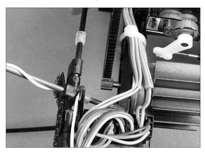
After confirming the point to which the pinion gear should be press fit onto the motor shaft, remove the motor from the frame. Then, following the instructions included with the motor, install the pinion on the motor shaft. The motor is now ready to install in the helicopter.
