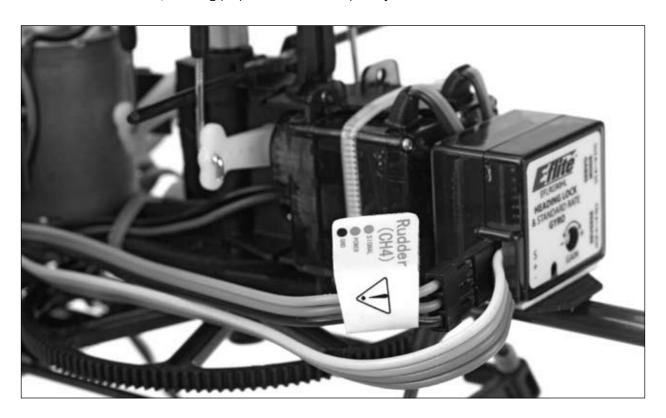
• If you will be using the remote gain control option for setting the gyro mode and gain from the transmitter, plug the gyro's auxiliary (AUX) lead into channel 5 of the receiver. Be sure that the lead is oriented properly so that it is plugged into the "signal" (like the orange wire on the servo leads) side of the receiver's pins.
