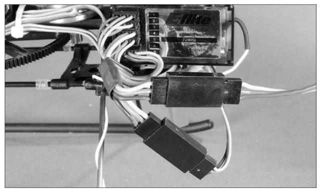
• To complete installation and wiring hook-up of the brushless ESC, connect the remaining JST male connector of the battery power lead Y-harness to the female JST connector of the 3-in-1 control unit. Be sure to then secure the battery power leads of the brushless ESC and 3-in-1 so that they cannot come into contact with the gears or any other moving parts, and so that you can readily access the remaining JST female connector for connecting the battery pack.
