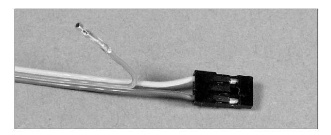
• Now that BEC power of the brushless ESC has been disabled, connect its receiver lead to one of the female connectors of the 3" Y-Harness (EFLRYH3). Next, connect the Throttle (Channel 3) receiver lead of the 3-in-1 control unit to the remaining female connector of the 3" Y-harness. Then, connect the male connector of this Y-harness to Channel 3 (Throttle) of the receiver.
