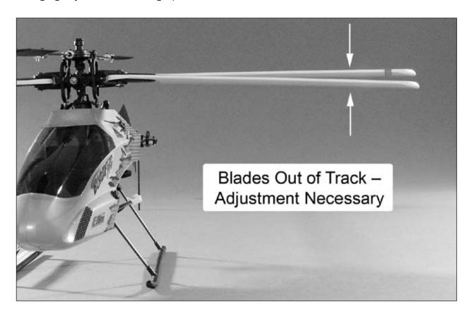
You can then power the helicopter down and increase the pitch of the low blade by turning its Pitch Control Link
