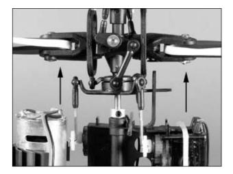
Again viewing the helicopter from the left or right side, move the right-hand stick forward and aft to check elevator pitch control. When the stick is pushed forward, the swashplate should also tilt forward.
