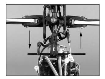
With the stick pushed right, the swashplate will tilt to the right.
