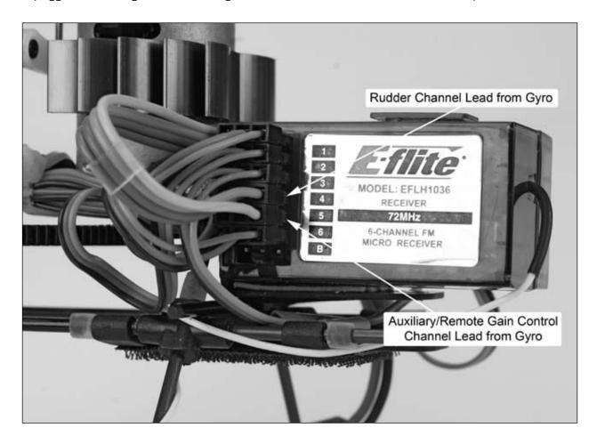
Note: It is important to secure the 3-in-1 rudder, gyro rudder and auxiliary channel leads so that they can not come in contact with the pinion and main gear, servo arms or motor case. We suggest using the cable/zip tie wraps included in the "Mounting Accessories & Wrench" package to secure the leads to the main frame.
