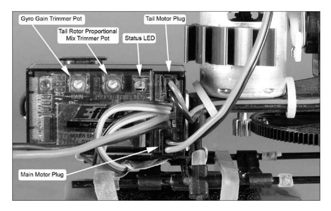
While each Blade CP Pro model is test flown at the factory with adjustments made to both the gain and proportional trimmer pots, further adjustment to these trimmer pots may be required based on the performance of the battery used, or preference and flying style of the pilot. However, before any changes to the trimmer pots are made, test flights will need to be conducted. Use the following check list for your first and all subsequent flights:
