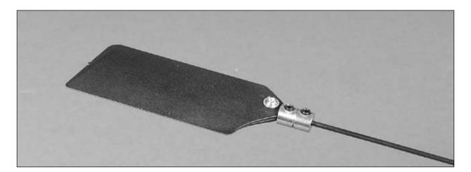
If, after the first few flights, you would prefer to have even quicker and more aggressive cyclic response, you can reposition the flybar weights so that they are closer in to the head/main shaft on the flybar. It is usually best to move the weights in only a small distance at a time before making each subsequent test flight, until you find the position at which you prefer the cyclic response most.
