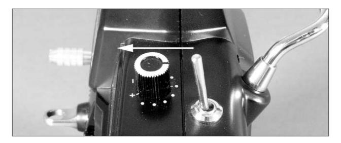
Note: When in the Idle Up/Stunt flight mode, even with the throttle stick all the way down, the blades and motors will continue to spin. You must use the Normal flight mode to safely turn off the motors. For safety, the 3-in-1 unit will not arm if the flight battery is plugged in and the flight mode switch is in the Idle Up/Stunt position.
