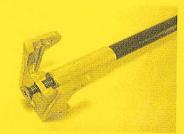
STEP 3: ATTACH THE MAIN BOOM TO THE BOOM MOUNT WITH THE 3X10MM FLATHEAD PHILLIPS SCREW. ALIGN THE LARGE FIN SO THAT IT IS POINTING UP VERTICALLY.
