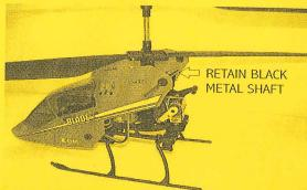
STEP1: REMOVE THE STOCK REAR BODY BY PULLING THE PINS OUT OF THE RUBBER GROMMETS. RETAIN THE BLACK METAL SHAFT TO MOUNT THE TAIL BOOM.
